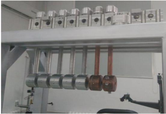
Figure 5: Alignment experiment with the test drift tubes.
