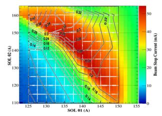
Figure 2: Beam stop current scan plot and rms norm. isoemittance areas (black lines), measured at March work point. It is possible to identify the almost monotonic emittance trend from lower right corner to left upper corner.
