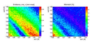
Figure 7: RFQ output beam parameters (mismatch and emittance) with the change of the lebt solenoids.
