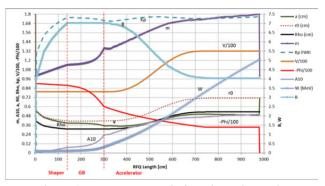
Figure 1: Parameters evolution along the RFQ.
