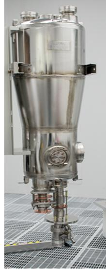
Figure 3: 72.75 MHz quarter wave resonator.
