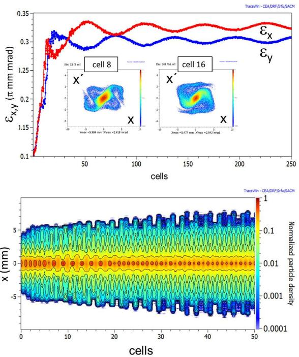
Figure 4: Top graph: rms emittances versus cell number for  $k_{0,x,y} = 120^\circ$ ,  $k_{x,y} = 70^\circ$  for Gaussian distribution with inserts showing phase space plots. Bottom graph: evolution of density (with contour lines) in  $x$  along the lattice.
