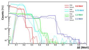
Figure 6: experimental and simulated neutron energy deposits in µLoM for different neutron incident energies.
