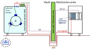
Figure 7: LIPAc vault and electronics area separated by a concrete wall for radiation shielding purpose.
