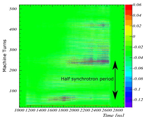
Figure 7: The fast recycler instability in the horizontal plane. The color scale represents horizontal motion, in arbitrary units. Shown is the first injected batch (1.6  $\mu$ s) for about 500 turns after injection. The incoming beam is not perfectly matched to the rf bucket here, and the instability is seen to occur at bunch length minima, and in the center and the end of the batch.
