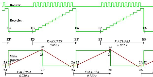
Figure 2: Relative timing of Booster, Recycler and Main Injector cycles for NOvA-era NuMI operation. Beam in each machine is shown in green, and Main Injector momentum in red. The start and end of cycle clock events for MI and Recycler are also shown.
