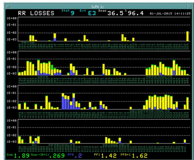
Figure 4: Loss around Recycler for 525 kW operation July 2015.
