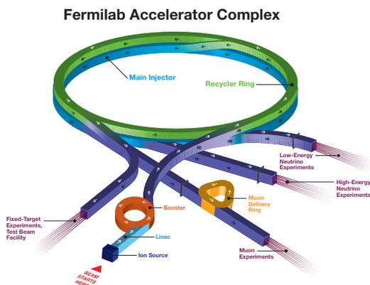
Figure 1: The Fermilab Accelerator complex in the NOvA era.
