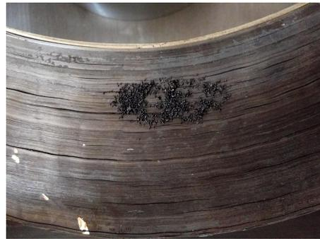
Figure 8: Local damage of type A MA core.
