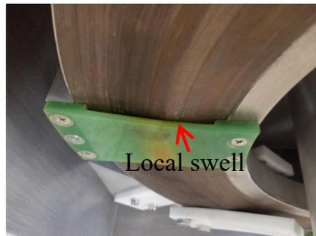
Figure 10: Local damage of type B MA core.
