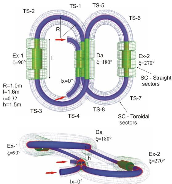
Figure 1: F8SR – Low-Energy Superconducting Magnetostatic Storage Ring.
