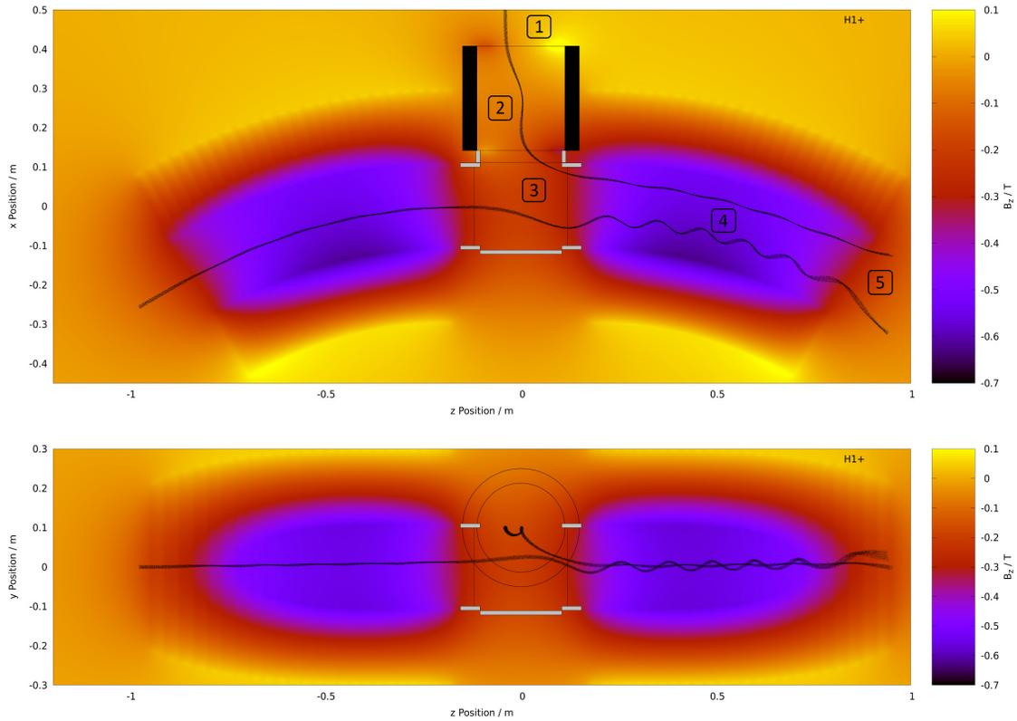
Figure 2: Looking on the beam path (upper picture from above / lower one from the side) of the ring beam and the injection beam. The magnetic field of the injection coil was  $B_{axis} = 0.326$  T, the offset of the injection channel 100 mm and the injection position  $x=508$  mm,  $y=100$  mm and  $z=-40$  mm.
