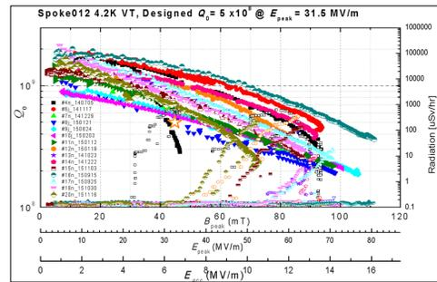
Figure 6: Vertical test results of Spoke012 cavities.
