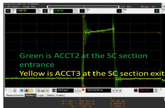
Figure 12: The transition rate of SC cavities.
