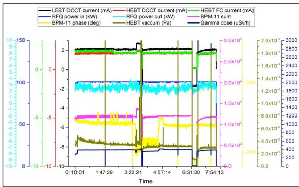
Figure 13: History record of 4MeV/1.7mA/CW/450min of injector-II.
