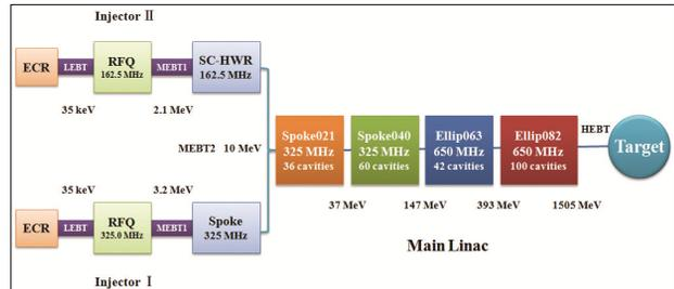
Figure 2: Layout of C-ADS linear accelerator.
