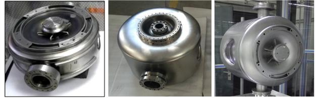
Figure 4: Spoke012, Spoke021, Spoke040 cavities.
