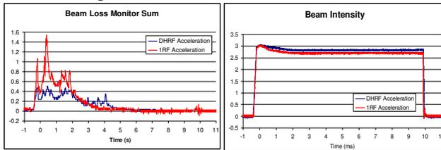
Figure 3: Beam loss (left) and intensity (right) with (blue) and without (red) DHRF cavity operation.
