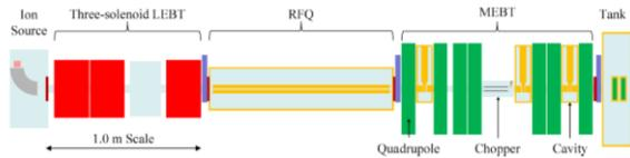
Figure 11: Arrangement of LEBT and MEBT.
