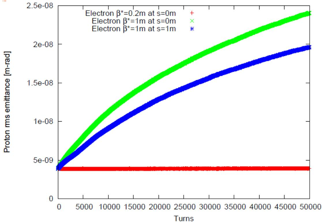
The proton beam emittance growth depends on electron IR optics choices.
