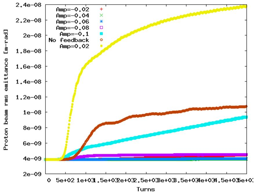
Proof-of-principle simulation run for the feedback system.
