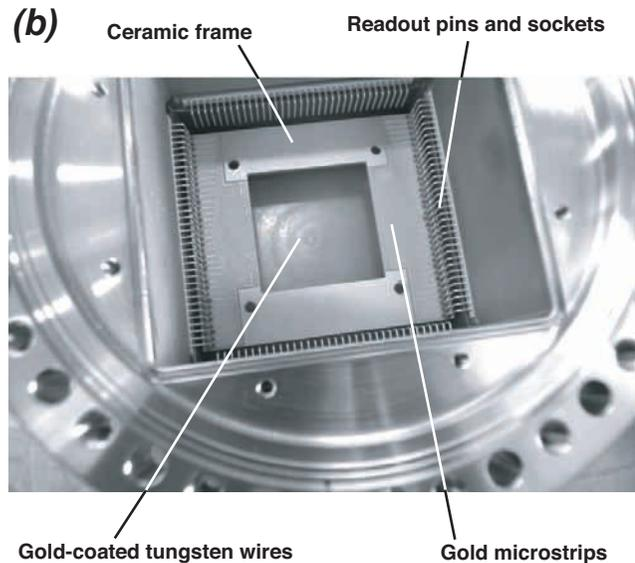
Gold-sputtered tungsten wires or carbon filaments diameter 5-30  $\mu\text{m}$  placed in UHV.
