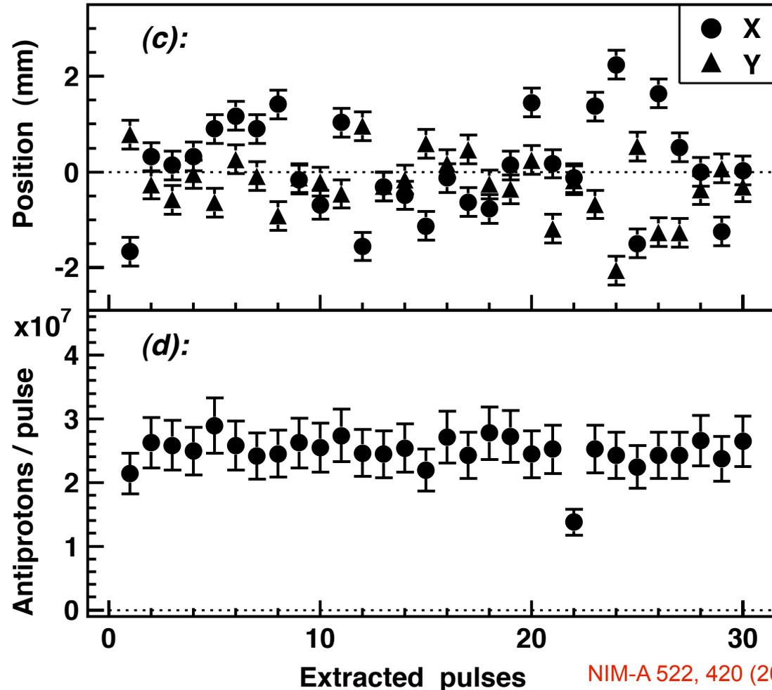
Clear profiles can be observed using the detection of secondary electron emission  $10^5 - 10^7$  particles/pulse
