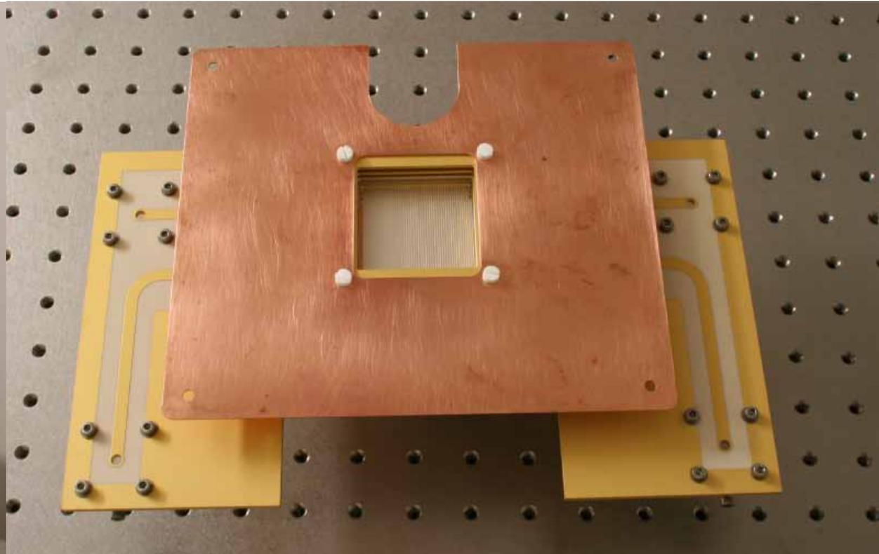
Four parallel 50-Ohm lines for effective impedance 12.5 Ohm allows fast switching of voltage potential
