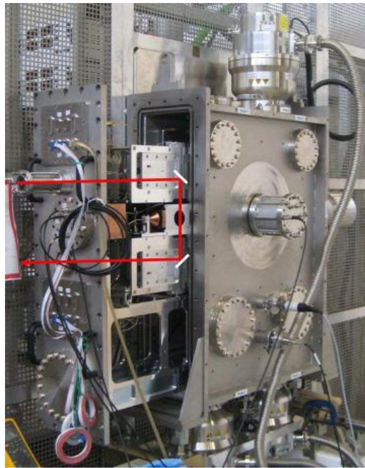
Optical beam path of the laser.
