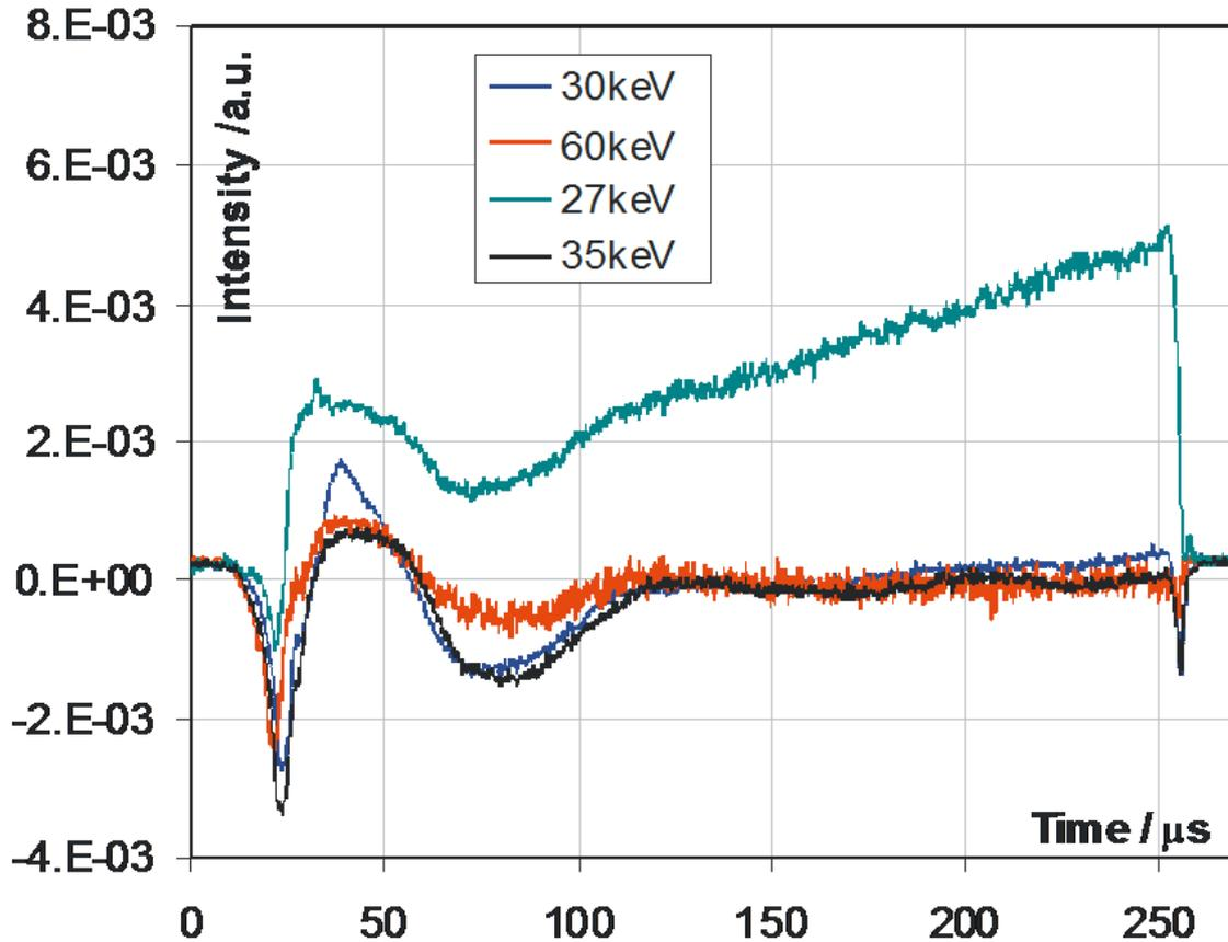
Detector chosen to negate signal at 35keV beam energy.
