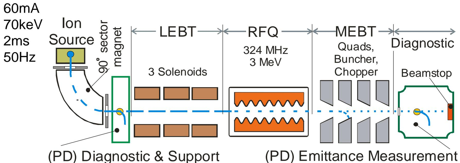
The beam profile monitor is placed in the first vessel downstream of the ion source and post acceleration system.
