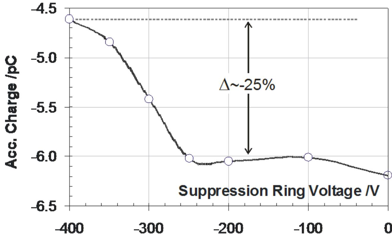
Variation of the suppression ring voltage to avoid penetrating others than photo detached electrons into FDC.
