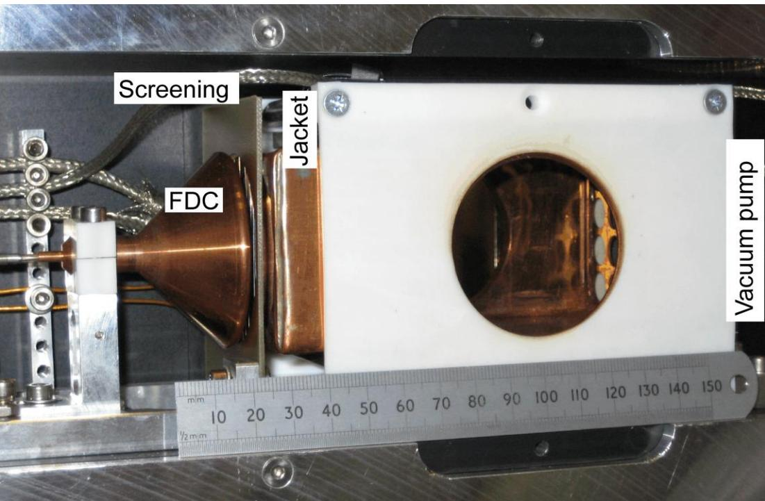
Blow up of the electron detector. Opening hole is 50mm in diameter.
