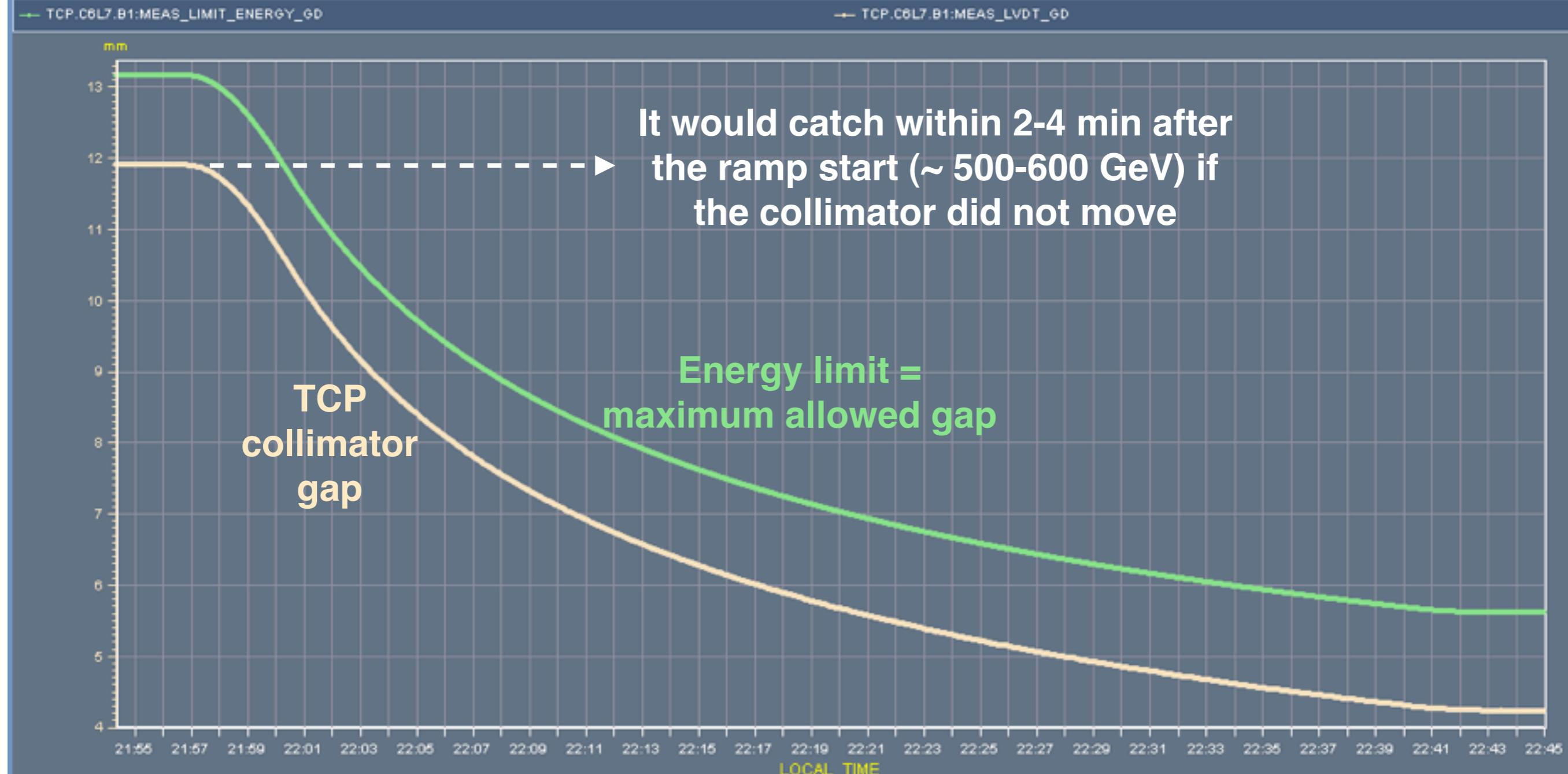
Redundant interlock, independent on trigger: it uses the safe machine parameters.
