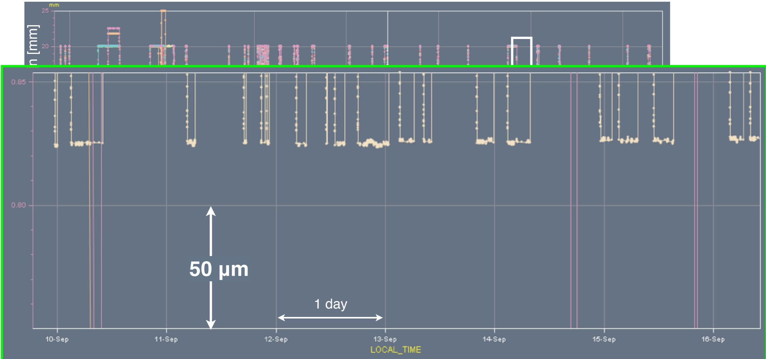
*Collimator settings are reproducible within a **few micrometers** over periods of several days!*
