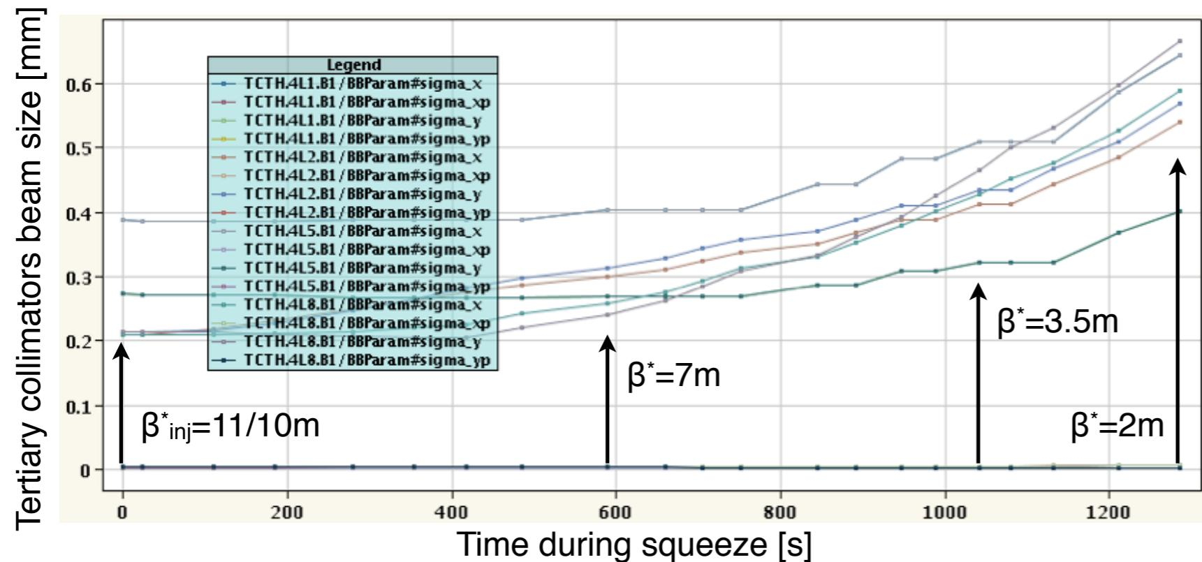
Beam size change at the **tertiary collimators** in the experimental regions during the betatron **squeeze** at constant energy.
