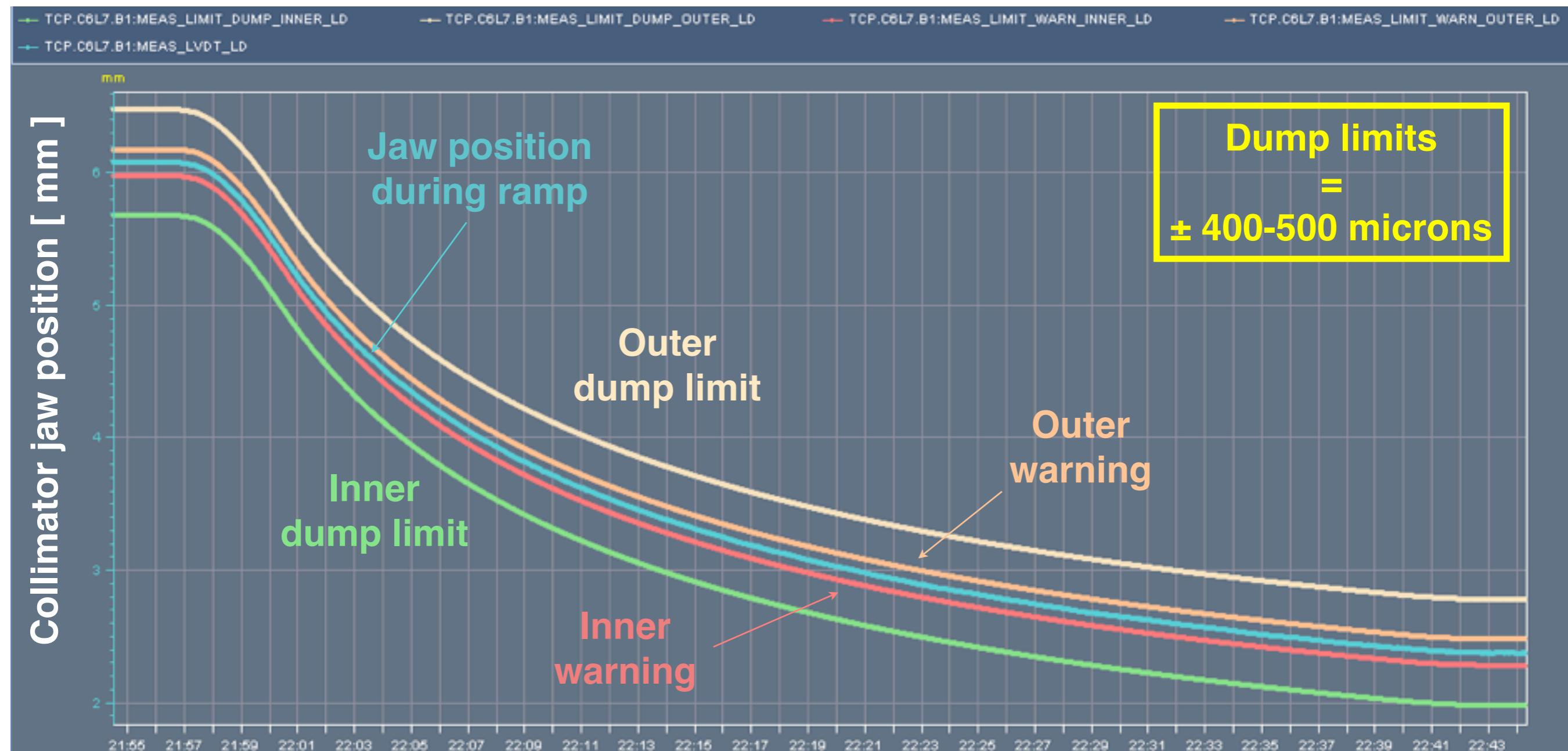
Limit functions (24 per collimator!!) are loaded for all ring collimators.
