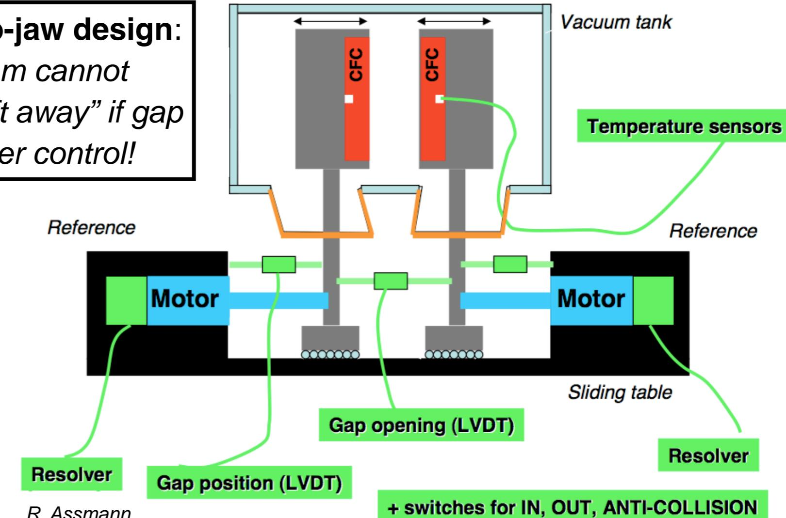
Settings: **4 stepping motors** for jaw corners - 1 motor for tank position.
