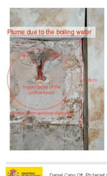
There are very clear signs of a strong **pitting corrosion** at the entrance of the proton beam. Such effects are very well known in nuclear power plants (cracks in the fuel cladding): the very hot (boiling) water carries more oxygen, thus allowing the Pb to change its oxidation state to higher values:
