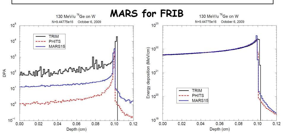
Pencil beam, uniform in R=0.03568 cm disc. Target  $W_{nat}$ , cylinder with R=0.03568 cm, L=0.12 cm
