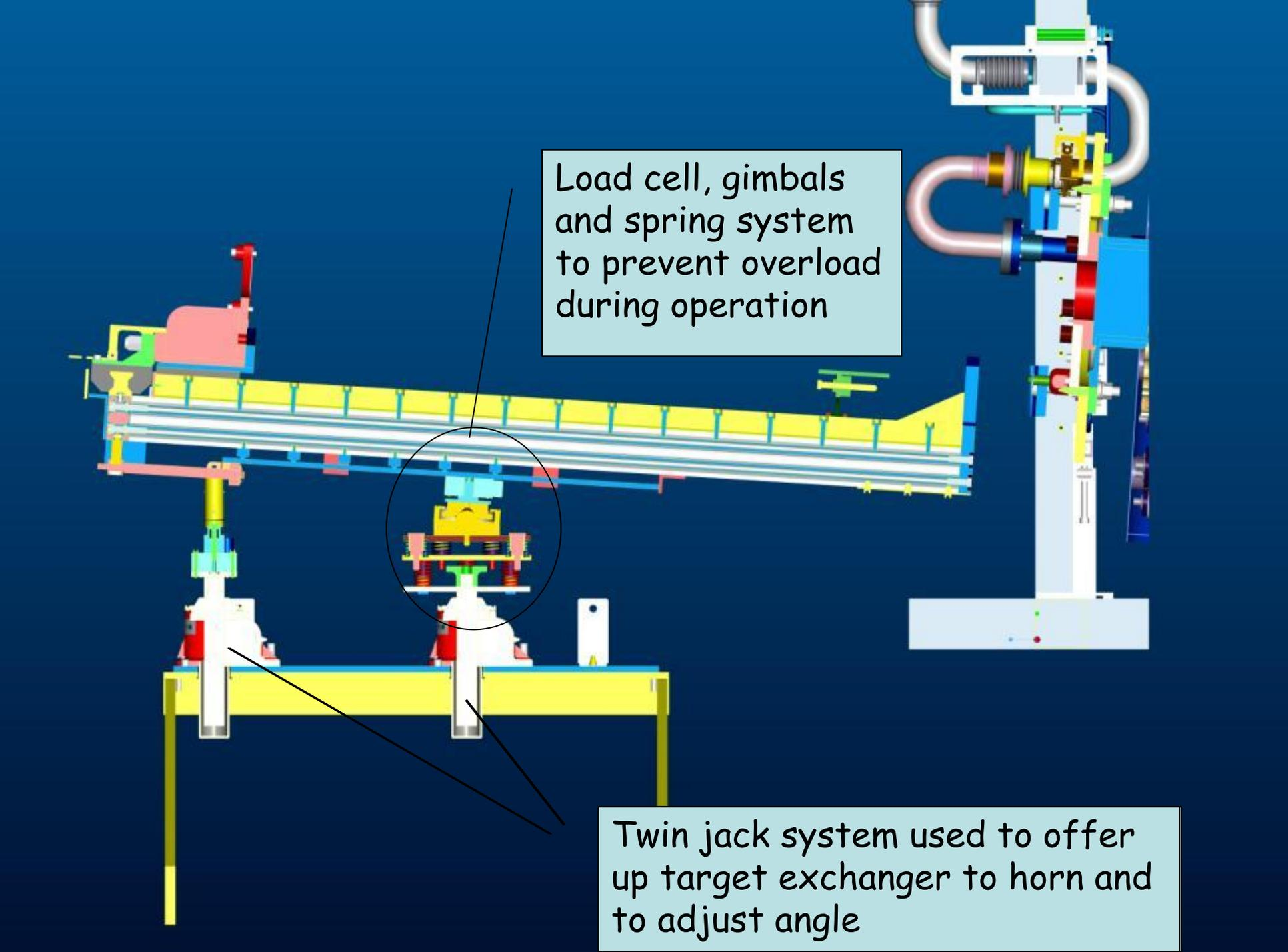
A 3D CAD model of a mechanical testing rig. The rig features a long, yellow, tapered beam supported by a twin jack system at the base. A circular callout provides a magnified view of the support mechanism, showing a load cell, gimbals, and a spring system. A second callout points to the twin jack system. The rig is mounted on a yellow table. On the right side, there is a vertical assembly with various pipes and components.
