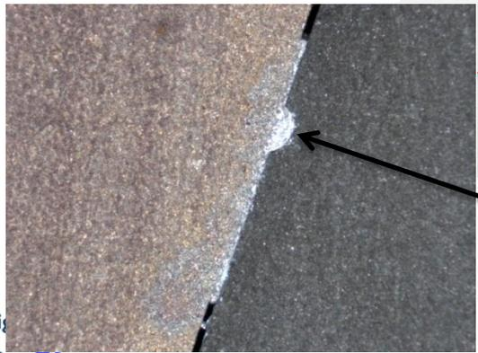
Aluminium intermediate layer, bonding temperature 550°C
