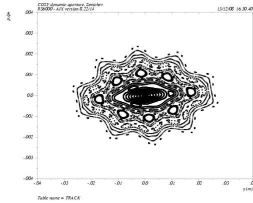
The vertical DA of the PAX lattice for monochromatic p-beam cooled by the Gaussian e-beam with  $\sqrt{r^2} = 6 \text{ mm}$  (a),  $\sqrt{r^2} = 3 \text{ mm}$  (b) and current 175mA
