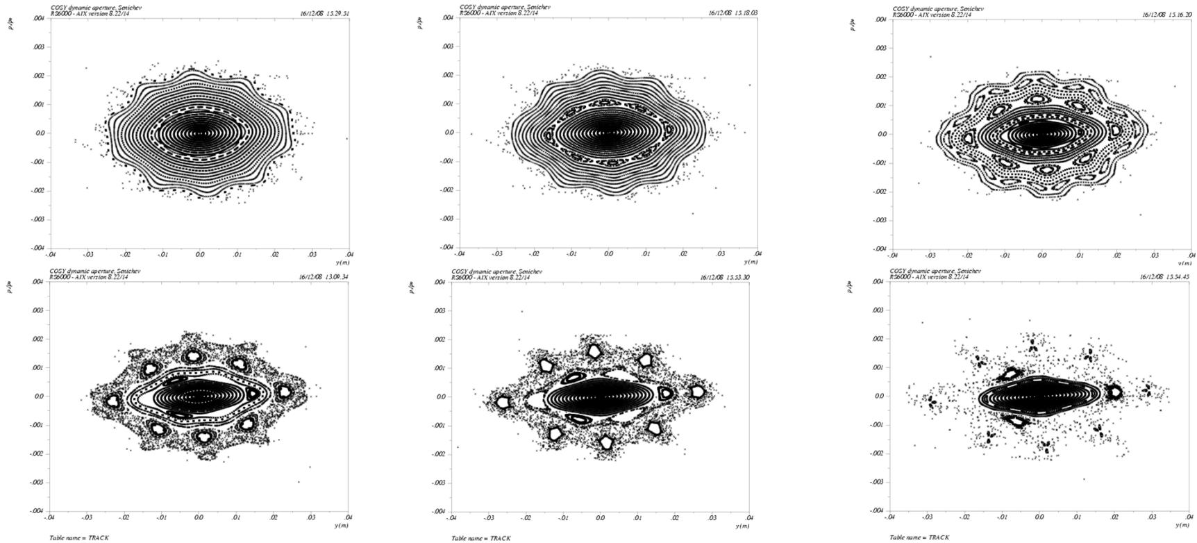
The vertical DA of the PAX lattice for monochromatic p-beam cooled by the uniform e-beam with  $\sqrt{r^2} = 6$  mm and current 175mA (a), 2 x 0.175 mA (b), 3 x 175 mA (c), 4 x 175 mA (d), 6 x 175 mA (e), 7 x 175 mA (f)
