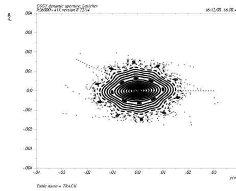
The vertical DA of the PAX lattice for monochromatic p-beam cooled by the uniform e-beam with  $\sqrt{r^2} = 6 \text{ mm}$  (a),  $\sqrt{r^2} = 3 \text{ mm}$  (b) and current 175mA
