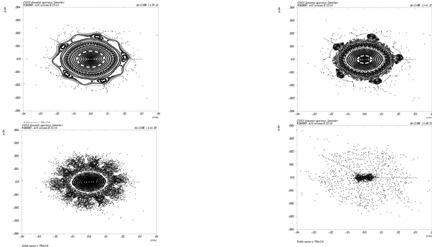
The vertical DA of the PAX lattice for non-monochromatic p-beam with  $dp/p = 1 \cdot 10^{-4}$ ;  $2 \cdot 10^{-4}$ ;  $4 \cdot 10^{-4}$ ;  $5 \cdot 10^{-4}$  calculated for the uniform e-beam distribution with dispersion 6 mm and current 175mA
