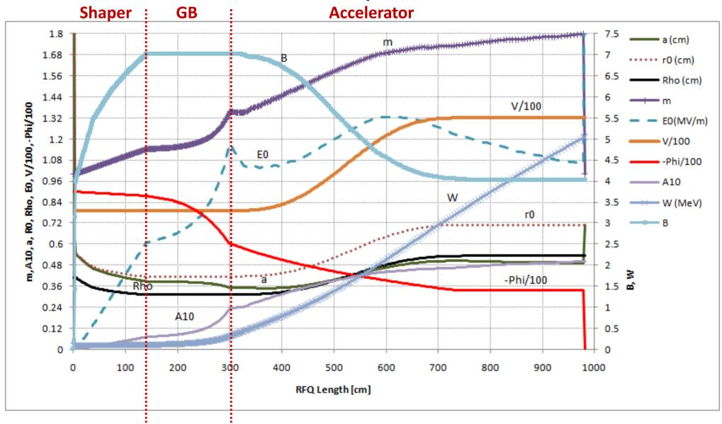
Deuteron Beam, Frequency=175 MHz, Current=130 mA, CW, energy from 0.1 MeV to 5 MeV
