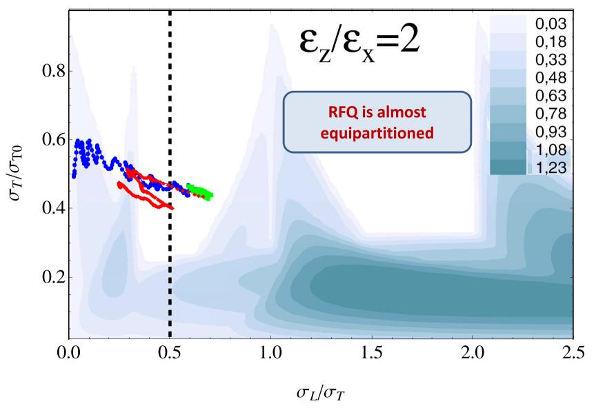
Stability chart, with overlapped the phase advance ratio for **Shaper**, **G.** Buncher, and **Accelerator**
