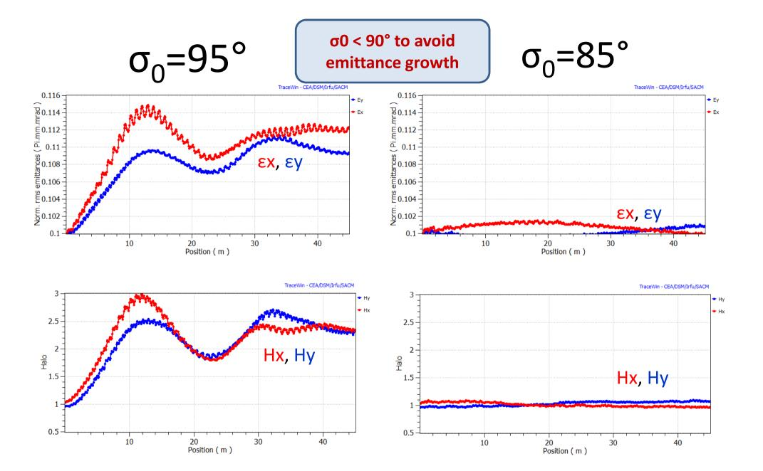
Example of FODO Channel  $\sigma/\sigma_0$ =0.85 Gaussian dist.
