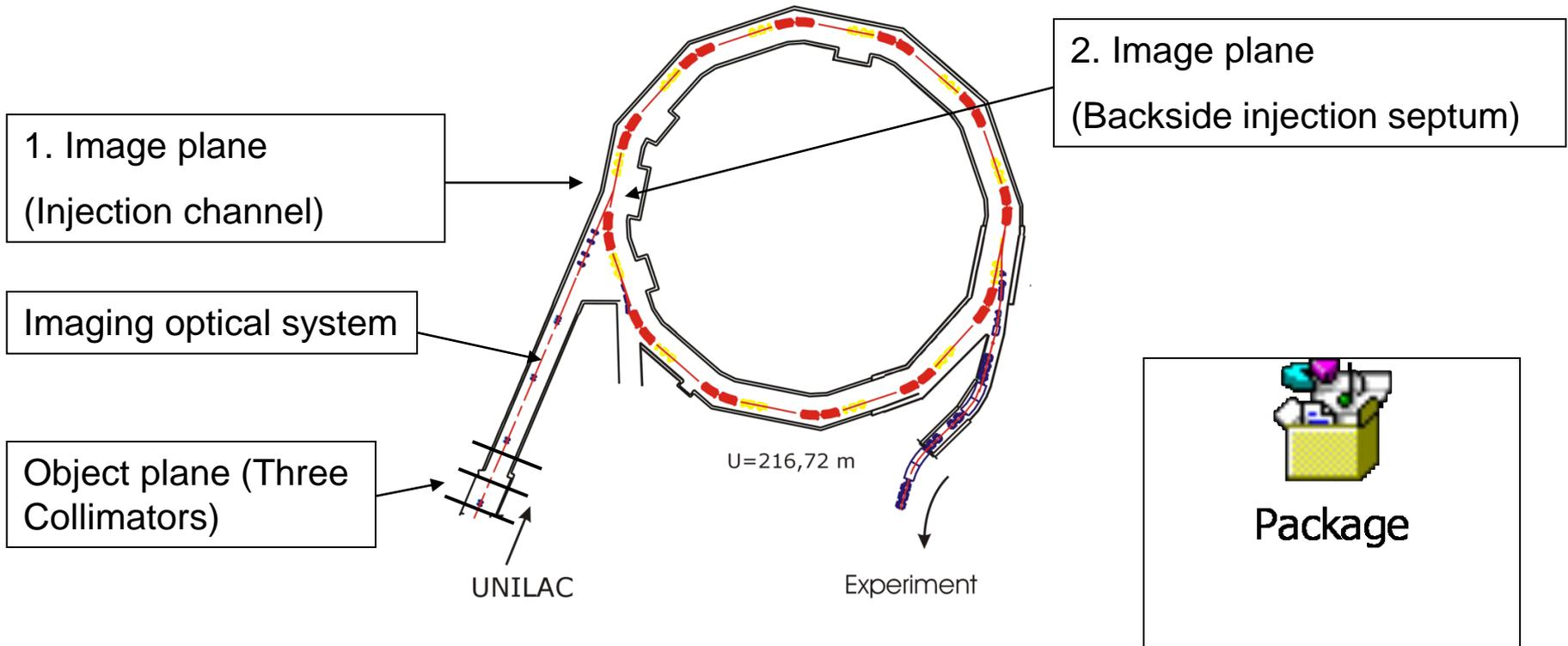
Imaging system from the collimator up to the injection channel and the backside of the septum
