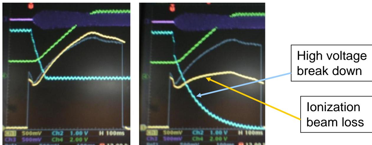
Gas desorption in the injection channel of the injection septum results in HV voltage break downs which again generates pressure bump and ionizes a large fraction of the beam after injection.
