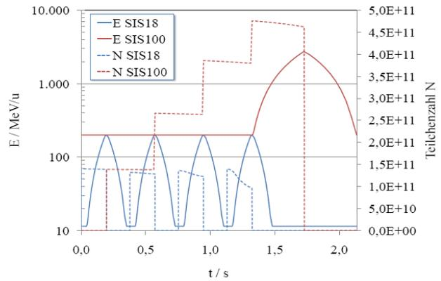
Ionization loss during stacking and acceleration in SIS18 and SIS100
