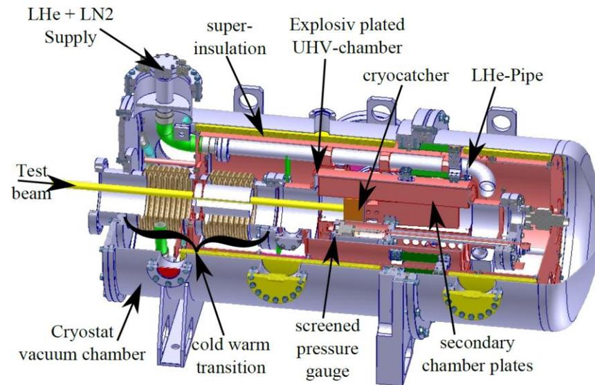
SIS100 cold, low desorption ion catcher (prototype)
