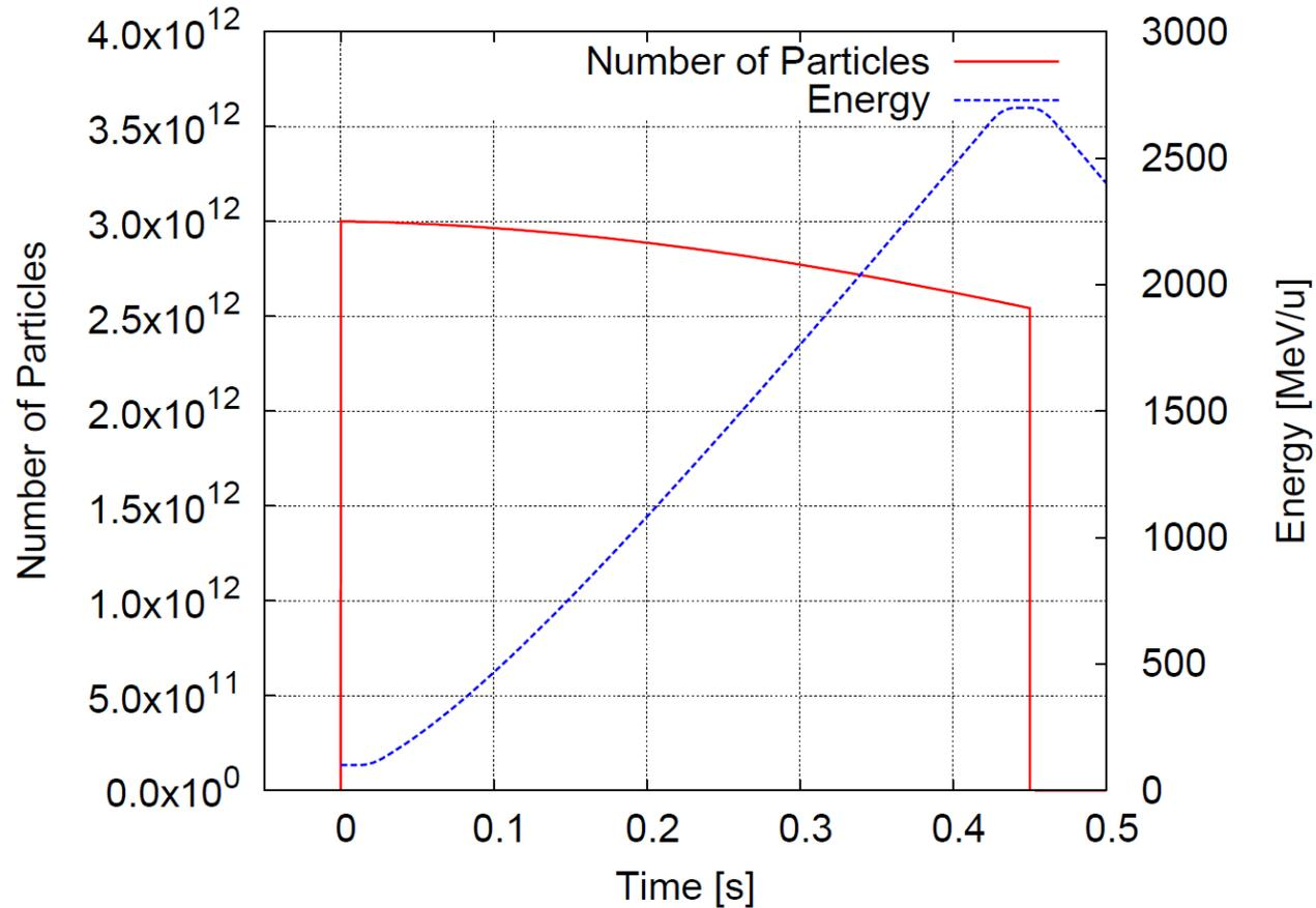
Ionization Beam Loss for U<sup>28+</sup>
