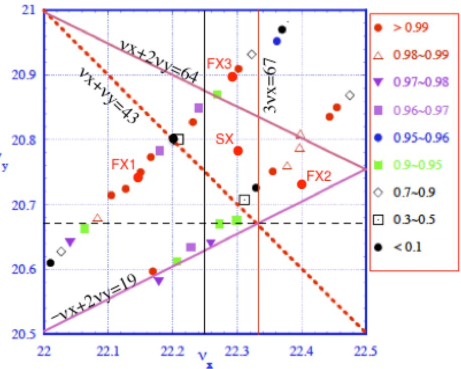
On the linear coupling resonance, we have large beam loss.
