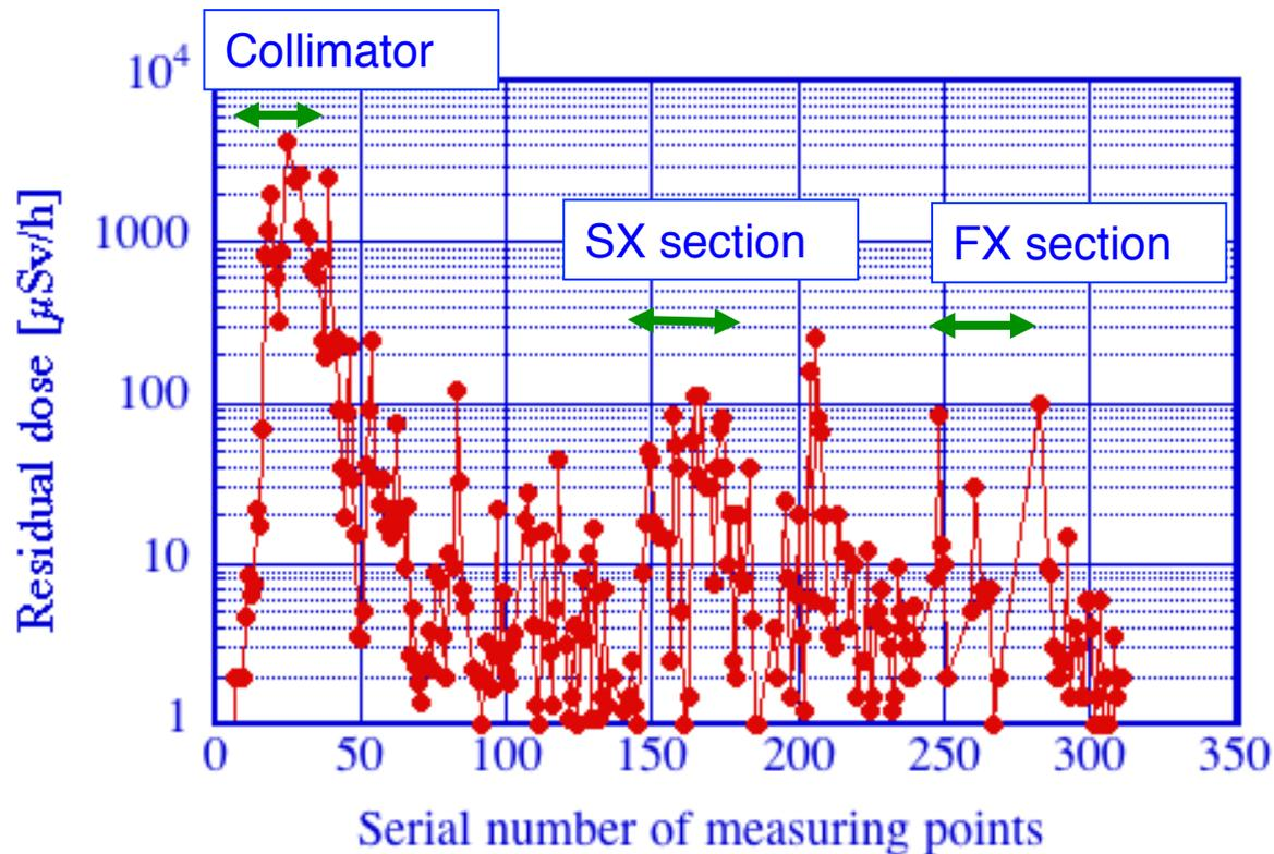
The residual activation in SX section 1 week after beam stop is less than 100  $\mu\text{Sv/h}$  on contact.
