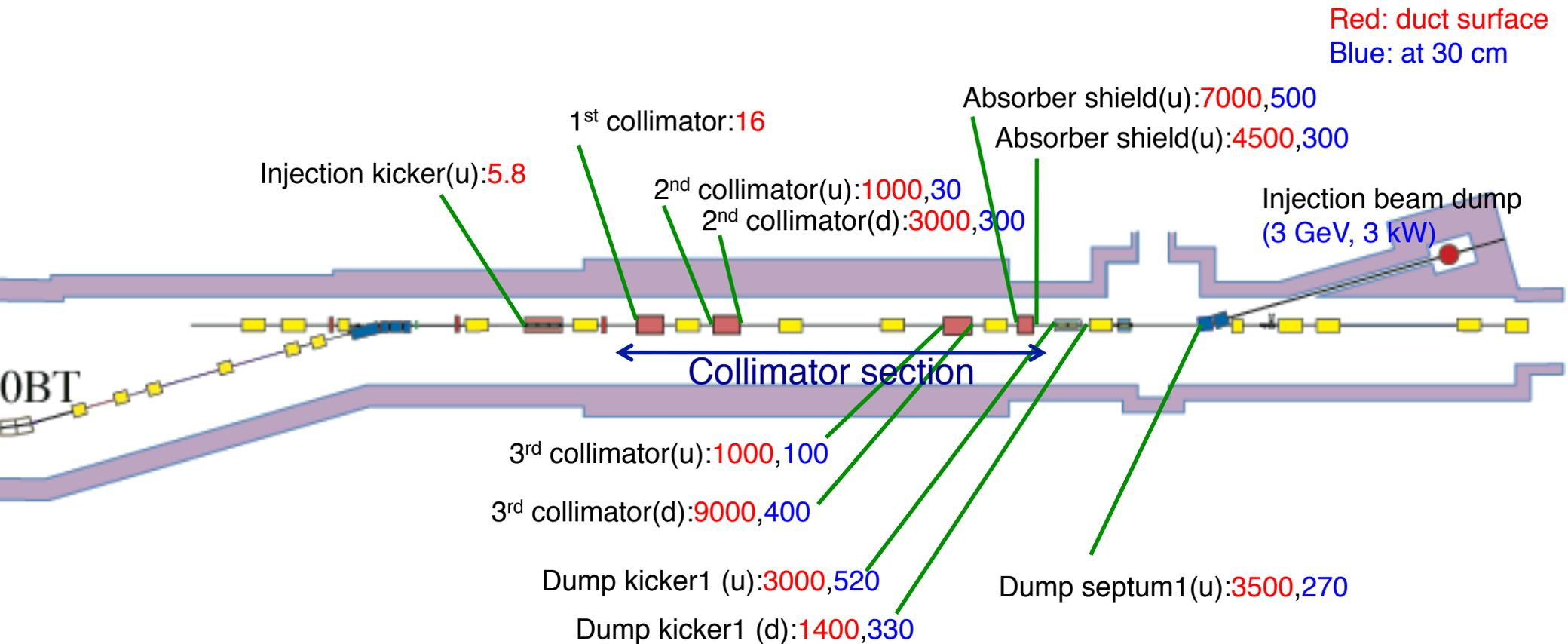
Injection dump system has high activation level because of the narrow aperture. We replace the beam ducts with larger ones in this summer shutdown.
