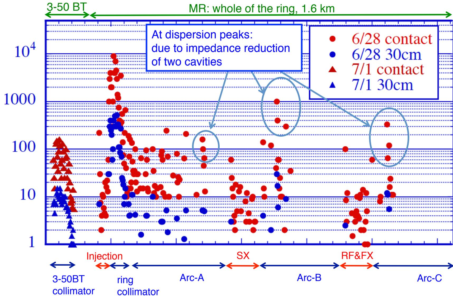
The aperture of the 3-50 BT collimator was set larger (~70 pi), because the installation of the additional shield was scheduled to start in the beginning of July. It can be used to reduce the loss in the ring collimators from the autumn run.
