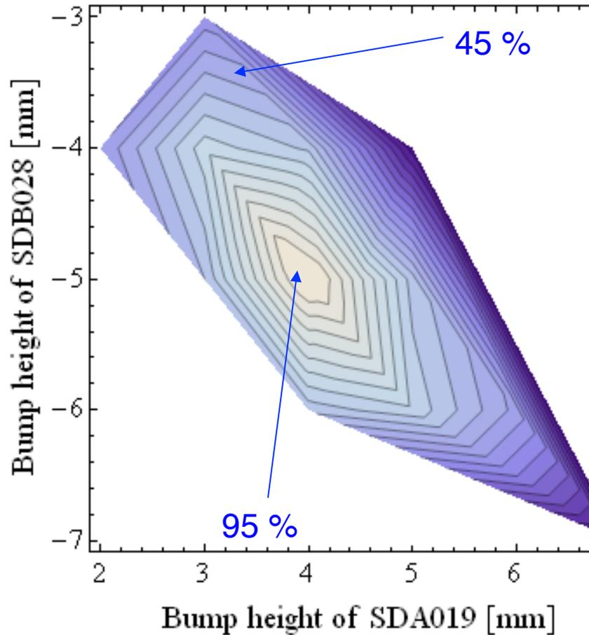
Measured beam loss on the linear coupling resonance for various pairs of bump heights.
