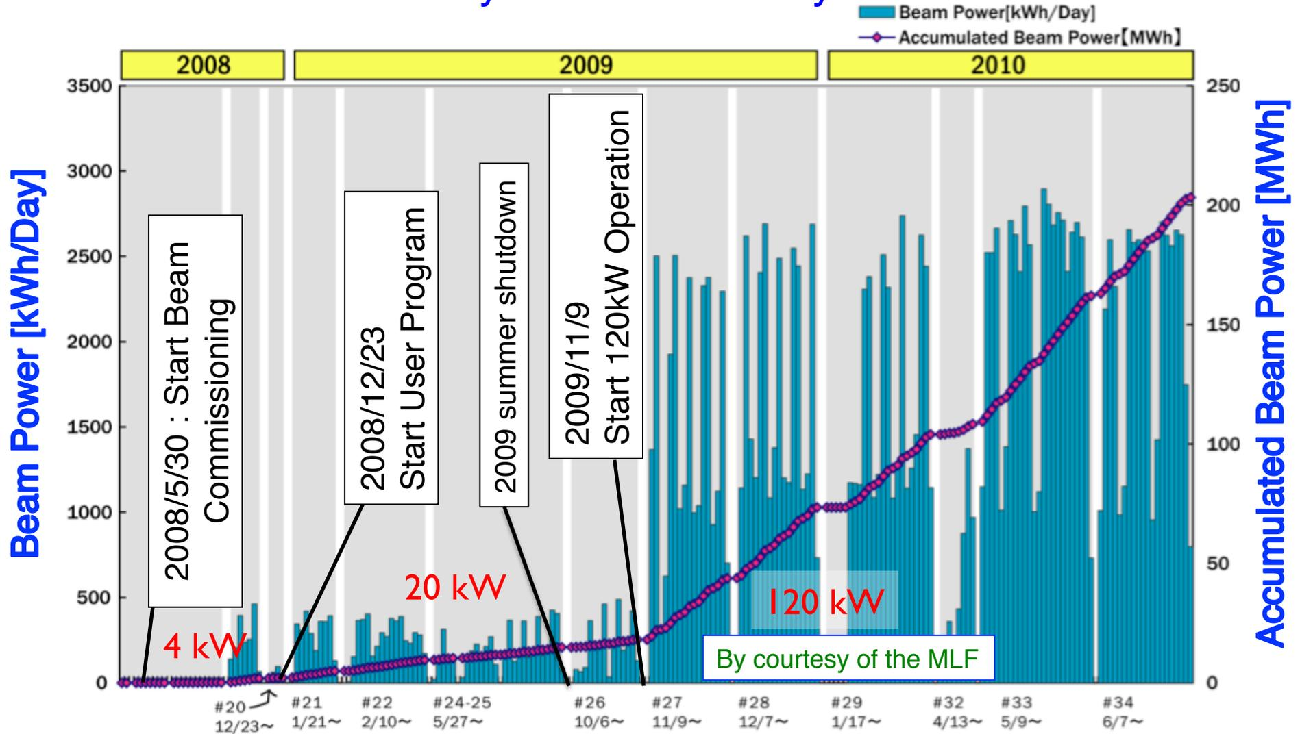
After the recovery of Linac-RFQ, high power operation of the RCS has become possible and 120 kW operation has started for the MLF users.
