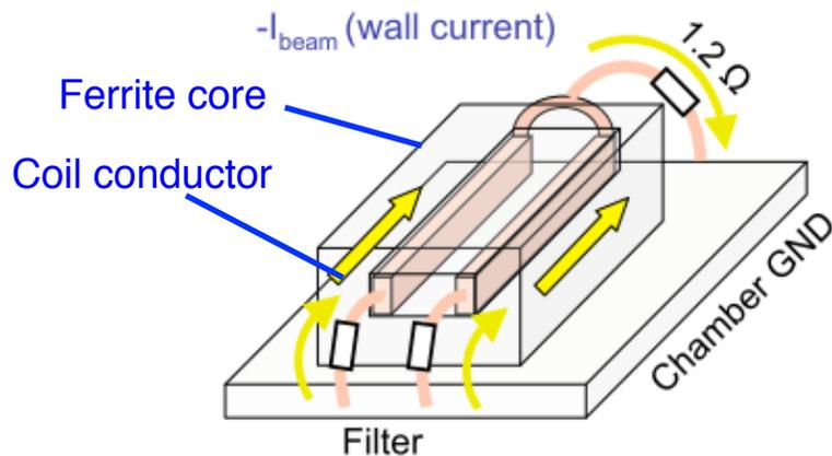
Ferrite core and coil conductor
