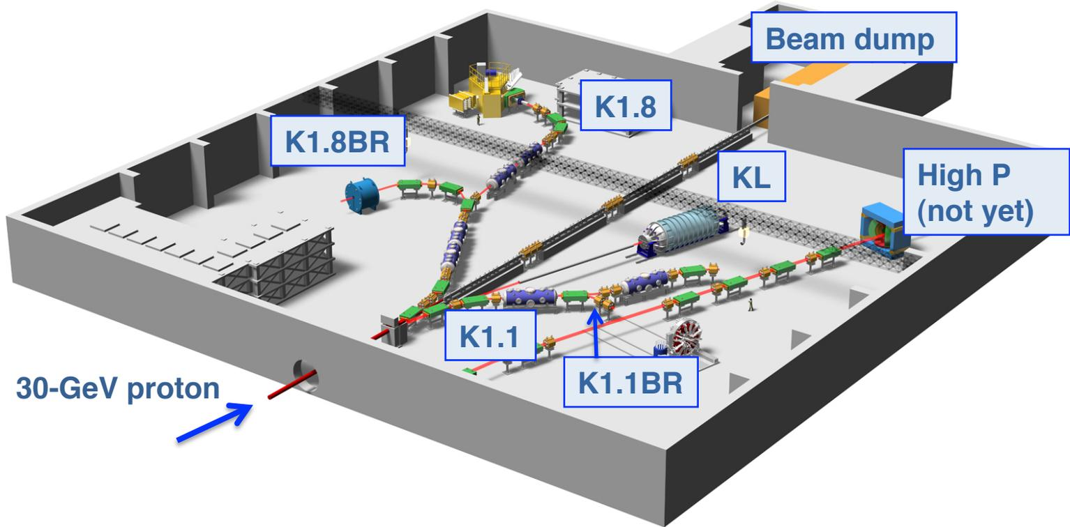
Layout of beam lines at the hadron experimental hall. Three beamlines (K1.8, K1.8BR, K1.1) are in operation. K1.1BR will be commissioned in October 2010.
