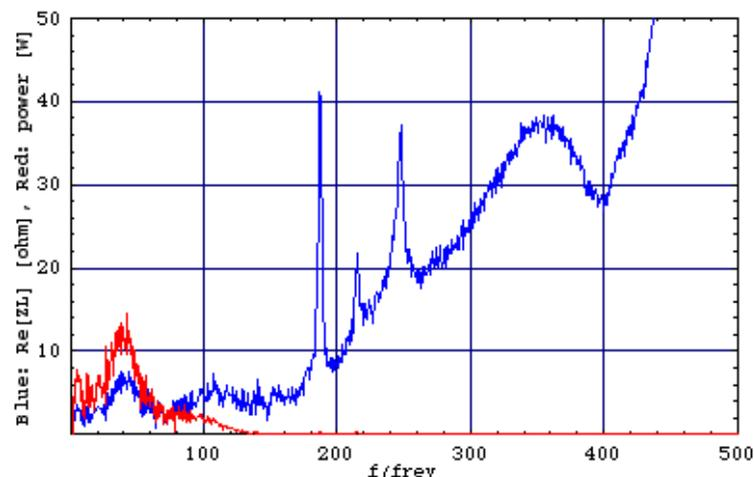
**Beam power spectrum:  $R_e[Z_L] \times I_B(\omega)^2$**
