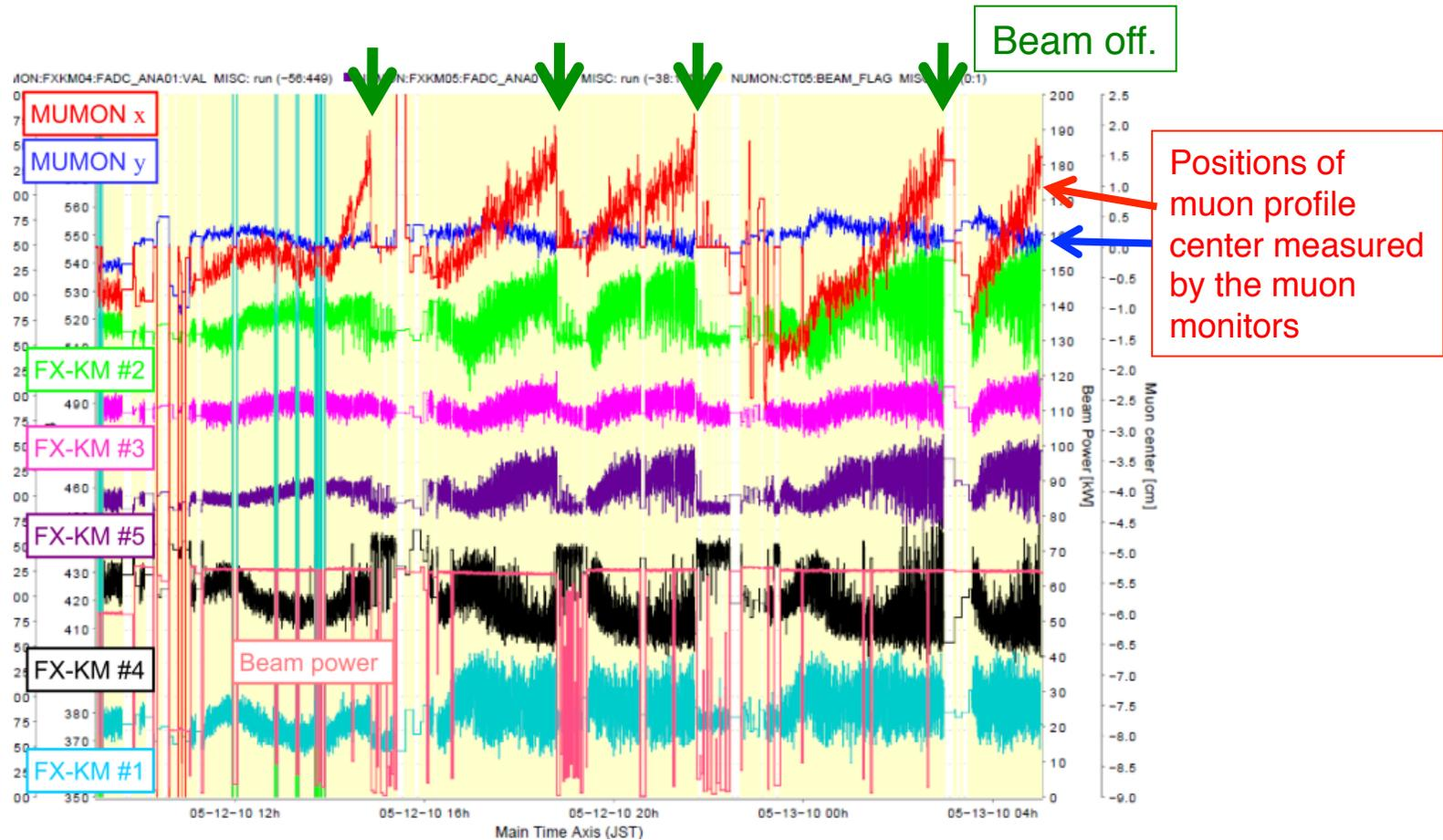
When the operation was resumed after ~30 min beam off, the beam came back to the initial position.
