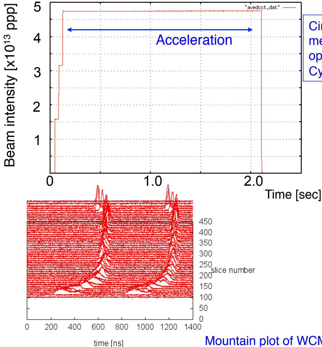
Circulating beam intensity measured by DCCT for 65 kW operation.
