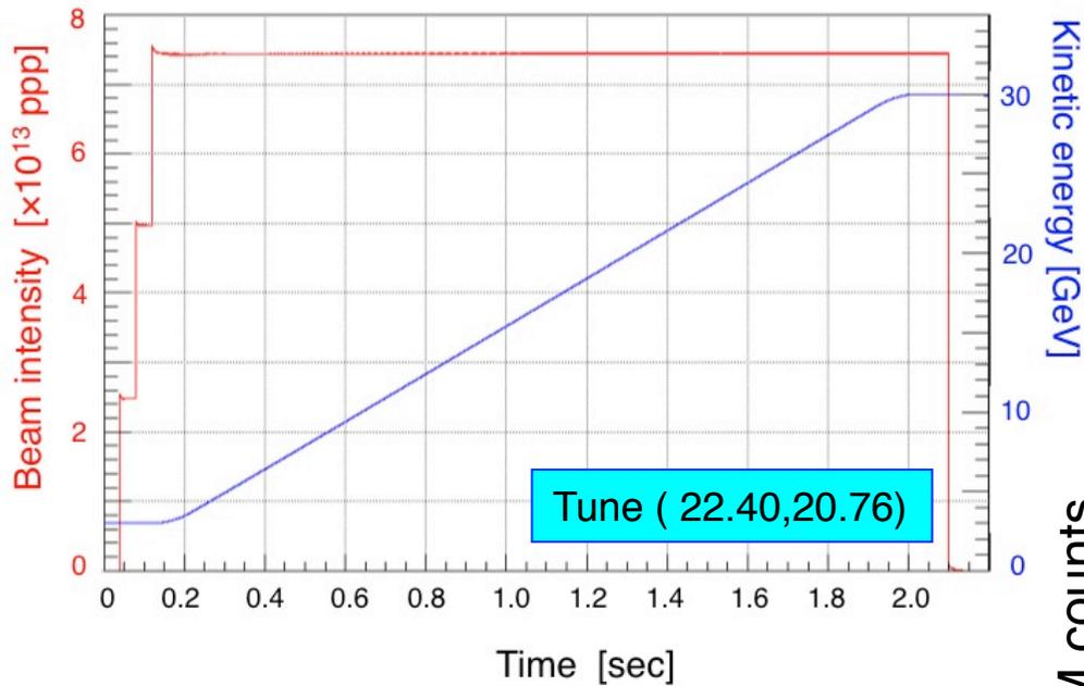
The extracted particles to the NU beamline is  $7.5 \times 10^{13}$  ppp:
