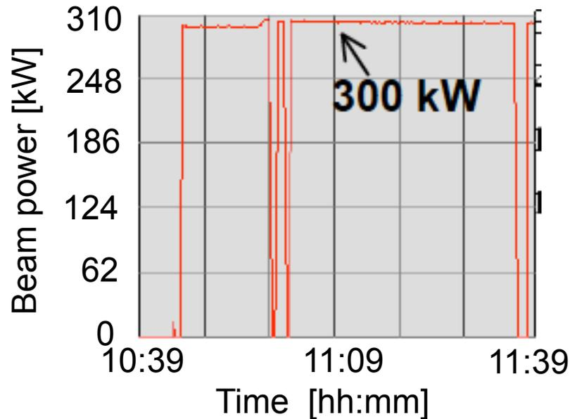
On Dec.10, 300 kW-1hours beam delivery from the RCS to the MLF was successfully demonstrated.
