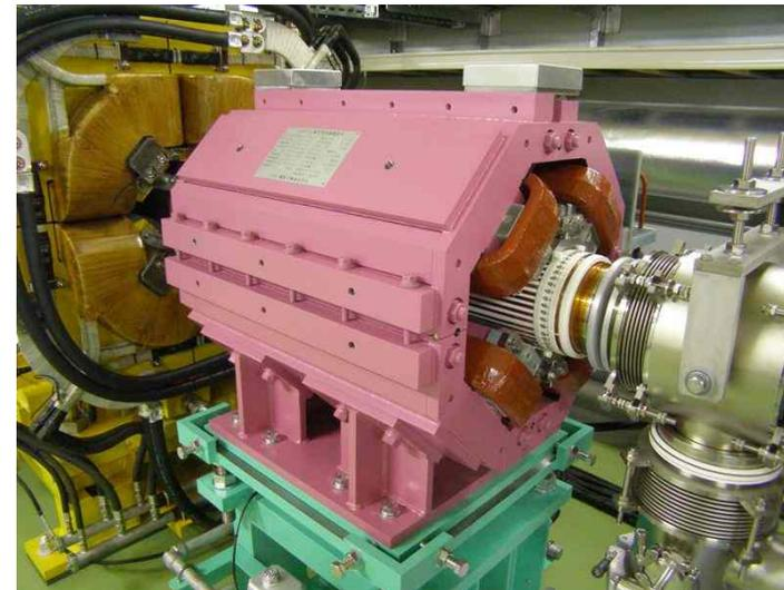
RQ: for ripple compensation ( $< 3$  kHz)
