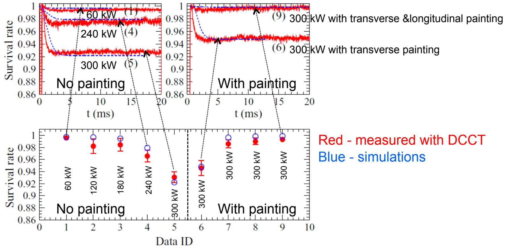
Intensity loss observed for 300 kW-equivalent intensity beam;
