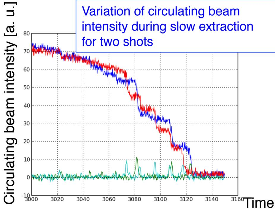
Because of the tune fluctuation, the circulating beam decreases in the step-like shape
