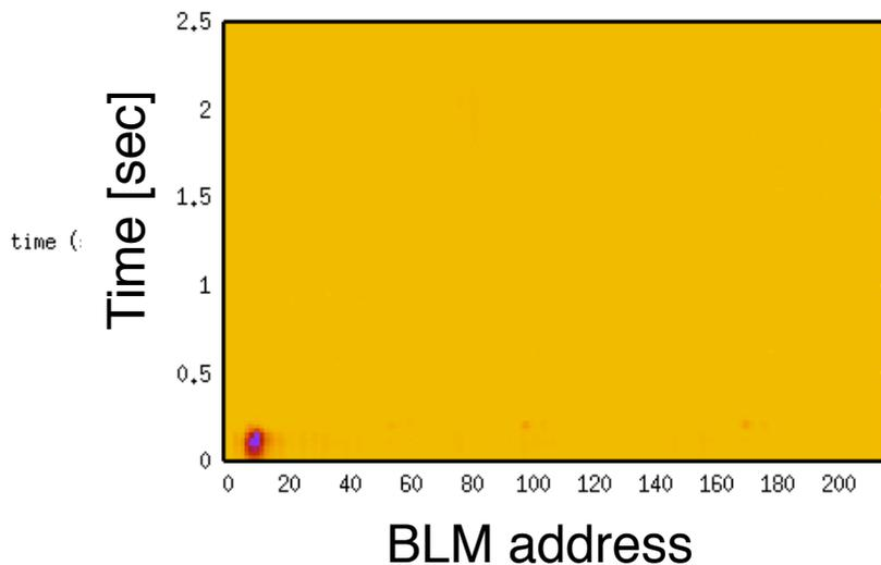
Typical injection loss is  $100 \sim 200$  W < present collimator limit 450 W
