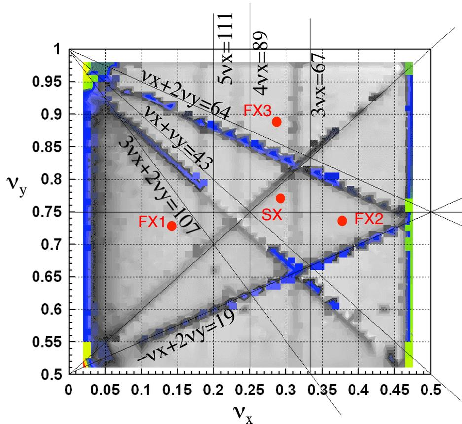
Measured results with 3 GeV DC beam of  $4e11$  ppb  $\times 1$  bunch ( 1% intensity )
