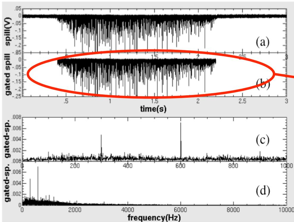
The spill has many sharp peaks, which come from fluctuation of tune due to current ripple of magnet power supplies.
