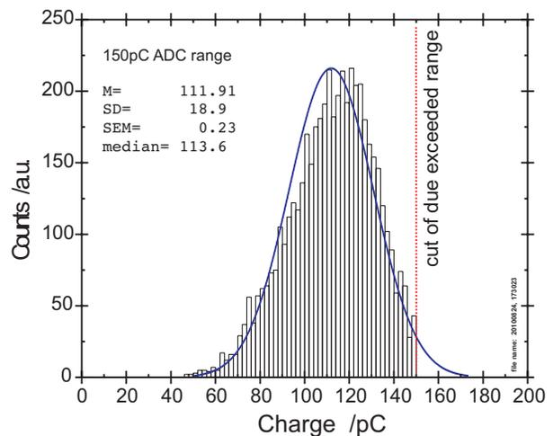
Figure 7: A typical distribution of measured charge, here shown as background (no laser,  $I = .335\text{ A}$ ,  $B = 89\text{ V}$ ,  $G = 155\text{ V}$ , total measurement time  $t = 203\text{ sec}$ , “B–cycle”).
