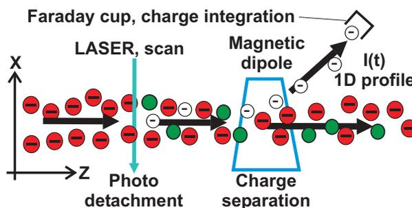
Figure 3: Basic principle of photo detachment ion beam diagnostics The  $H^-$  ions get neutralized by laser light. The diagnostics is in general a three stage process: detachment, charge separation and detection.
