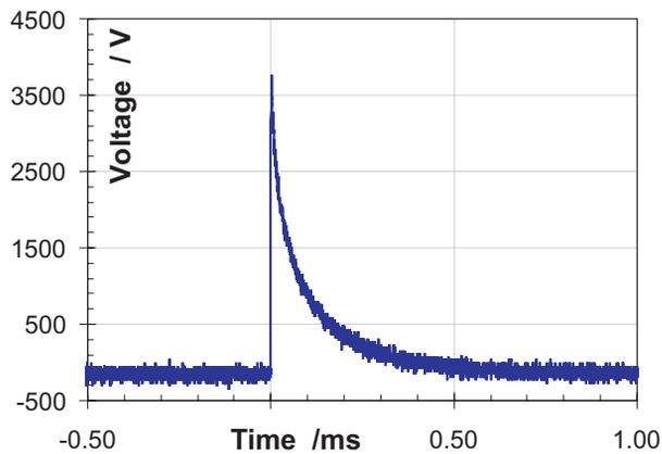
Figure 8: High voltage pulse, measured with a 1000:1 probe between BNC vacuum feed through coming from the FDC and ground outside the vessel.
