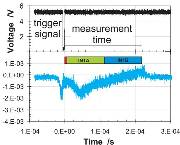
Figure 6: Triggering of the electronics and integration cycles of the ADC. Between the rising edge of the trigger and the start of the integration is a delay of  $6.3\mu\text{s}$ . The lower scope trace shows a typical background signal ( $\propto$  voltage drop on  $50\Omega$ ).
