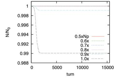
Figure 2: Beam loss rate for the intensities, 0.5, 0.6, 0.7, 0.8, 0.9, 1.0 times of the design bunch population,  $N_p = 4.17 \times 10^{13}$  in RCS, where  $\varepsilon = \varepsilon_x + \varepsilon_y = 100\pi \mu\text{m}$ .
