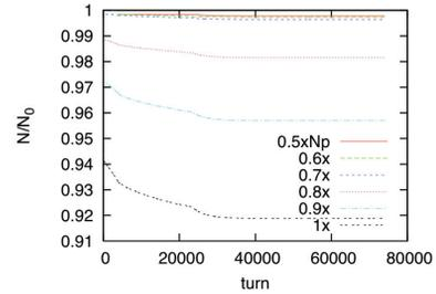
Figure 7: Beam loss rate for the intensities, 0.5, 0.6, 0.7, 0.8, 0.9, 1.0 times of the design bunch population,  $N_p = 4.17 \times 10^{13}$  in MR, where  $\epsilon = \epsilon_x + \epsilon_y = 100\pi \mu\text{m}$  in RCS injection.
