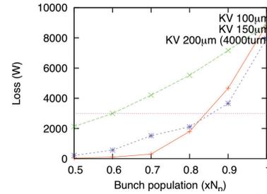
Figure 8: Beam power loss as a function of intensity in MR. The repetition is 0.45 Hz. The loss for  $\epsilon = 200\pi \mu\text{m}$  is integrated only up to 4000 turns.
