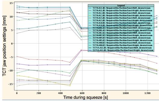
Figure 4: Settings generated for the TCT jaws in all IRs during the squeeze, taking into account (1) the settings of Table 2, (2) the beam-based orbit positions and (3) the beam size variation during the change of optics.
