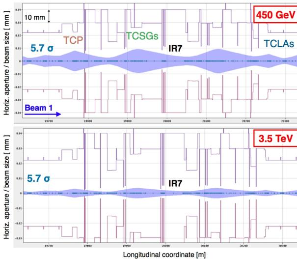
Figure 3: Horizontal aperture, collimator jaw positions (vertical bars) and  $5.7\sigma$  beam envelope at injection (top) and 3.5 TeV (bottom) in the betatron cleaning (IR7) from the LHC on-line model application [4].
