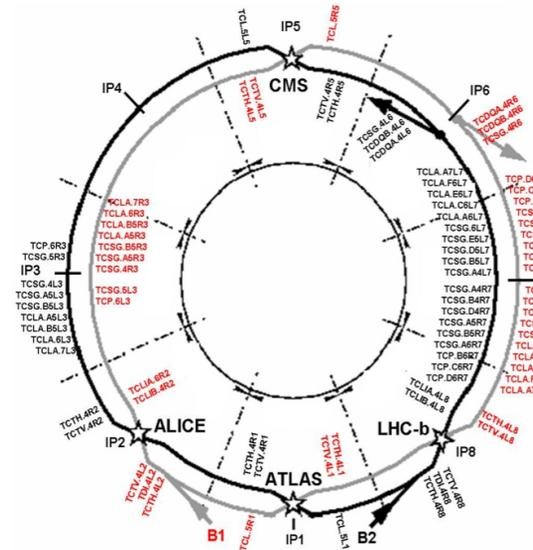
Figure 1: LHC layout with collimator locations [2].
