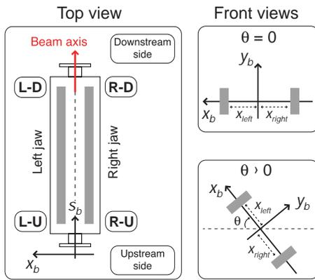
Figure 2: Schematic layout of an LHC collimator. Each jaw is moved with two independent stepping motors. Six linear variable differential transformers (LVDTs) measure the jaw corner positions and the collimator gaps at each jaw extremity. Four resolvers monitor the motor steps for a fully redundant position survey [3].
