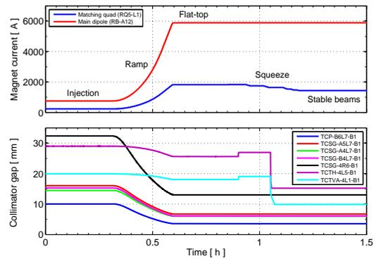
Figure 5: Operational cycle for a selected number of collimators. Measured magnet currents (top) and collimator gaps (bottom) versus time are given for a typical LHC fill.
