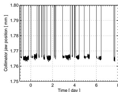
Figure 7: End-of-ramp settings for one TCP jaw as a function of time over 9 days. The fill-to-fill reproducibility with all the LHC equipment active is of a few  $\mu$ m, confirming the results of [5] in the real accelerator environment.
