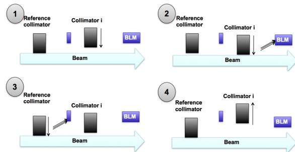
Figure 6: Scheme of the collimator setup procedure [8].
