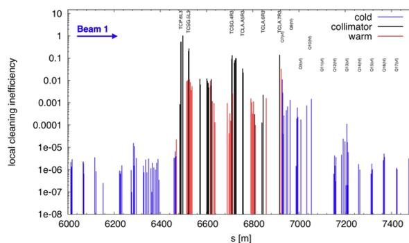
Figure 10: Momentum loss map for beam 1 at 3.5 TeV.
