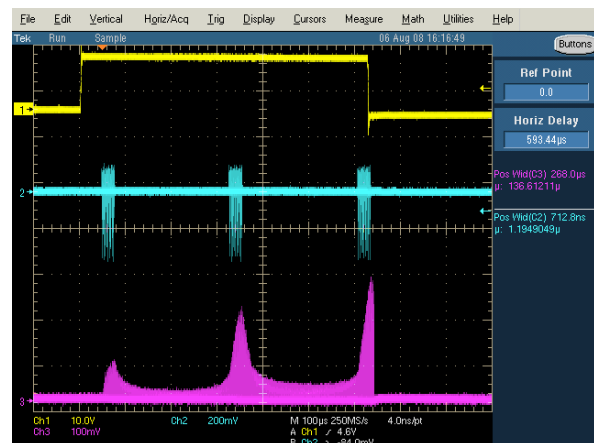
Figure 2: Beam gate (top trace), Linac micropulses (middle trace) and PSR circulating current (bottom trace) obtained during pulse-stacking demonstration.
