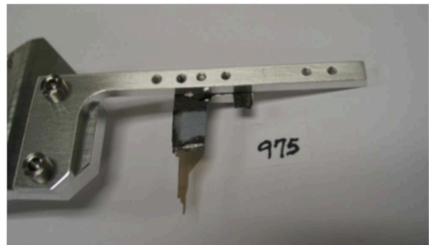
Figure 7: An example of a fractured foil substrate on a third-generation foil bracket.
