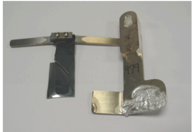
Figure 3: A failed second-generation foil and bracket. This foil lasted for a few hours at \sim 840 kW beam power. (Figure reproduced from Ref. 3.)
