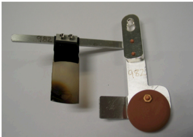
Figure 2: A used second-generation foil bracket. The beam power in this case was only 400 kW, so this foil and bracket show very little damage. (Figure reproduced from Ref. 3.)
