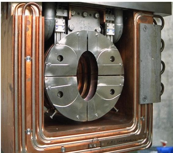
Figure 4: Segmented asymmetric collimator with readout of the four segments for measuring the currents.
