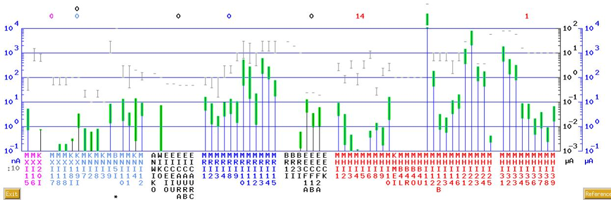
Figure 6: Beam losses display showing a reference with the actual losses as green or red change to this reference.
