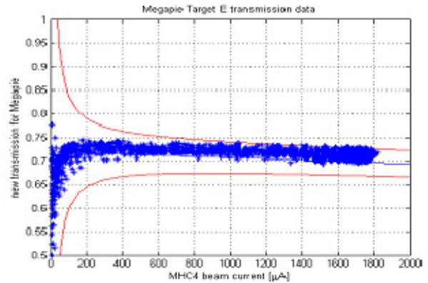
Figure 5: Validity window for the Target E transmission.
