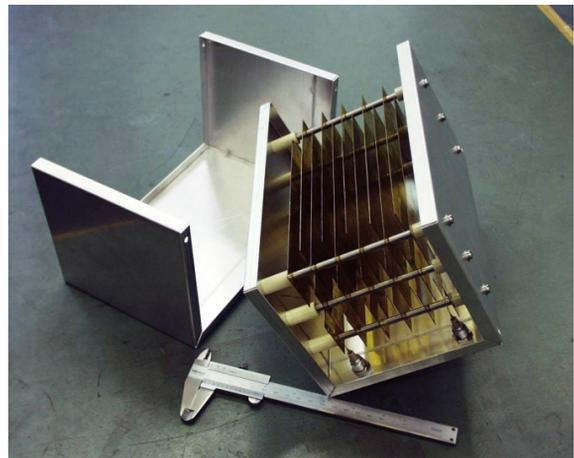
Figure 2: Ionization chamber for measuring beam losses.
