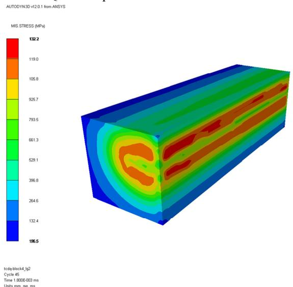
Figure 2: distribution of dynamic stresses calculated with AUTODYN®.
