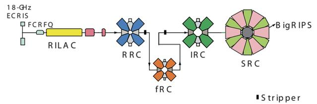
Figure 2: Acceleration scheme for uranium beams using two strippers.
