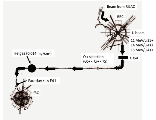
Figure 4: Schematic of experimental setup used for measurement of cross sections of e loss and e capture in RIBF beamlines.
