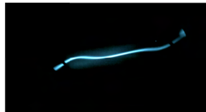
Figure 6: Electron projection for the horizontal profile affected by the proton beam.
