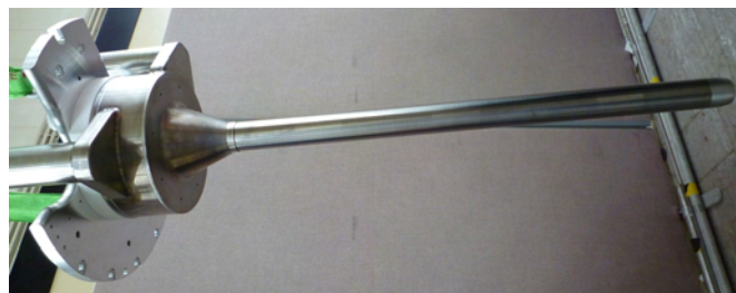
Figure 8: Completed target ready for integration with horn.
