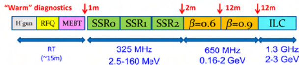
Figure 2: Project X CW linac baseline RF configuration.
