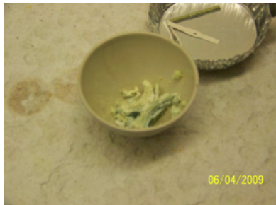
Figure 9: Oxidation of irradiated Ta at 1100°C.
