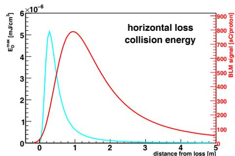
Figure 7: The comparison of longitudinal distributions of energy deposit in the coil and the BLM signal outside the cryostat.
