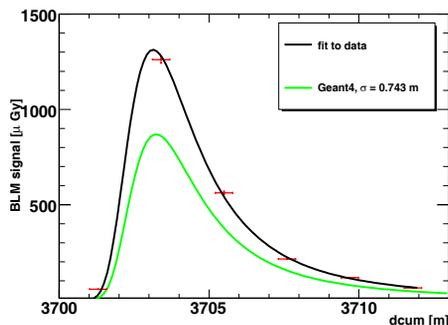
Figure 5: The BLM signal during a beam-induced quench of the MB magnet. Green line shows simulated signal, black line is a fit to the measurements. The quench has been provoked by about  $2 \cdot 10^9$  protons with an energy of 450 GeV.
