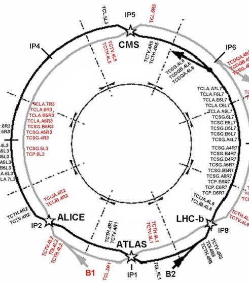
Figure 1: Sketch of the layout of the present phase-I collimation system. Beam 1 (beam 2) collimators are shown in red (black). [7].
