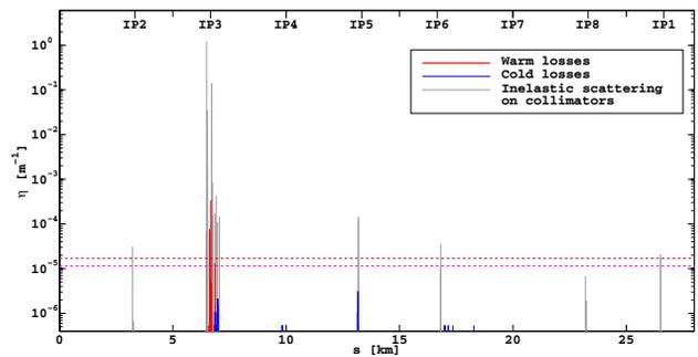
Figure 5: Cleaning inefficiency in beam 1 for a horizontal beam halo. In total 19 million particles were simulated. The red (purple) line marks the quench limit at 7 TeV/c for nominal (ultimate) intensity and a beam life time of 0.22h.
