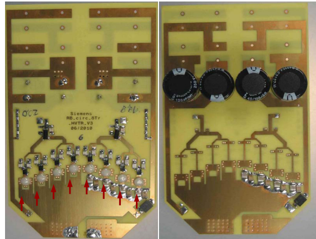
Figure 2: 20kW RF module with SiC devices (red arrows).
