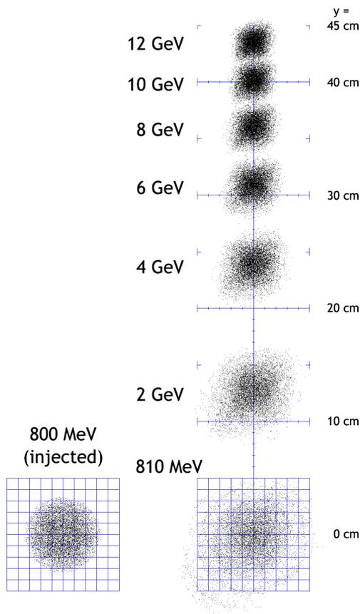
Figure 6: Acceleration of the 150 mm.mrad beam in real space, showing vertical motion and the increase in size of the beam as it matches to the nonlinear equilibrium phase space of the magnets over the first few MeV after injection.
