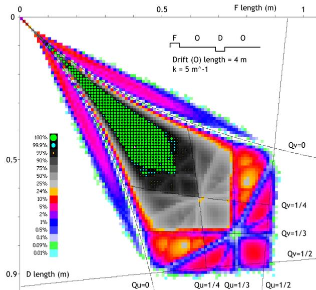
Figure 7: Effect on beam transmission of the lengths of the F and D magnets in the FODO cell. Magnetic fields are kept constant so this varies the total amount of focussing. Cell tune lines in the  $u$  and  $v$  skew planes are shown.
