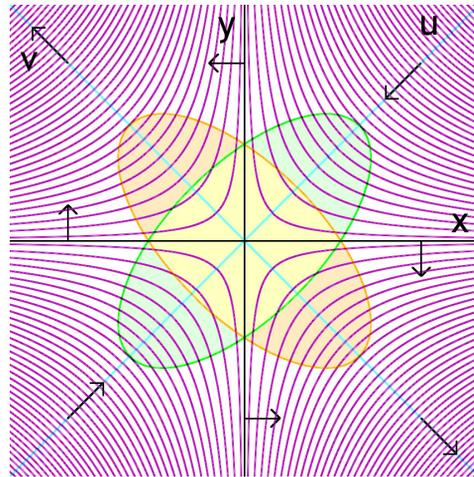
Figure 2: Skew focussing in the vertically-scaling FFAG field. The purple field lines cause the focussing forces (black arrows) along the  $u$  and  $v$  axes, giving beam cross sections that vary between the two elliptical shapes shown.
