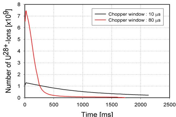
Figure 4: First experiments with  $U^{28+}$  in SIS18 in the year 2001. Ionization of the beam ions in local enhanced pressure regions which were created by ion induced desorption caused an almost completed loss of the beam.
