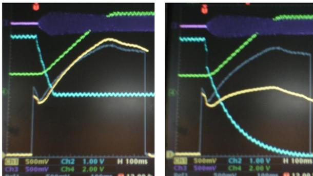
Figure 8: Beam current (yellow) over a machine cycle in SIS18. The blue line shows the voltage of the electrostatic injection septum. The green curve indicates the magnetic field cycle. In the right picture, a high voltage brake down has generated a strong local pressure bump just after injection. The locally enhanced pressure creates major beam loss by charge exchange over the whole cycle.
