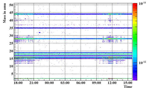
Figure 1: The residual gas spectrum in a synchrotron is changed by desorbed gases. During high current operation (left and right), additional components appear with a density comparable with the background components. The gap in between indicates the time of low intensity operation.
