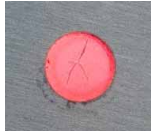
DAST crystal cracked after a few seconds of exceeding 60 C locally (500 \mu\text{m} spot size, 200 kHz)
