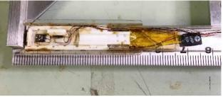
Figure 3: Photograph of a Hall sensor array, which can measure three-component magnetic fields along the z-axis. The second and fourth Hall sensors from the left are used to measure the  $B_{\text{und}}$  component.
