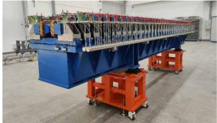
Figure 4: The THz undulator for SXFEL.
