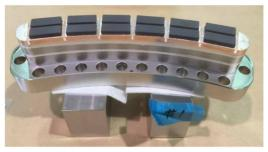
Figure 3: HOM damper with 12 ferrite bars.
