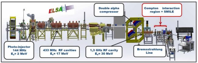
Figure 1: Layout of the ELSA Accelerator.
