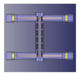
Figure 1: Top down view of stripline with vacuum vessel hidden.
