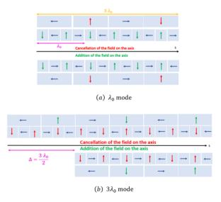
Figure 1: Configuration of magnet magnetization.
