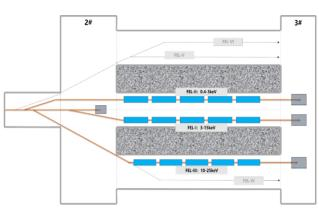
Figure 1: Undulator system at the SHINE. Main dump is located at the beam switch-yard system in the tunnel 2, and the other three dumps are at the downstream of the undulator systems in the tunnel 3.
