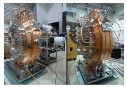
Figure 1: RF cavity with the compact HOM-damping structure.
