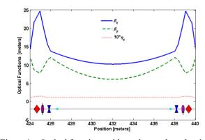
Figure 1a: Optical functions without the quadrupole tripole in the 12-meter-long straight.
