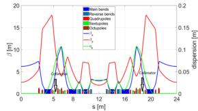
Figure 1: The lattice functions and magnet layout of the HALF storage ring (with collimator positions marked).
