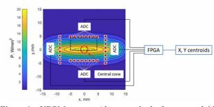
Figure 1: sXBPM concept (detector pixels shown overlaid on the X-ray power density distribution 26 m away from a single EPU in the non-canted configuration).
