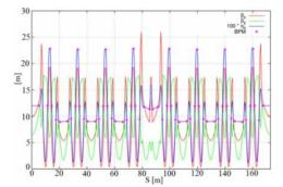
Figure 1: Optical functions of the double mini- $\beta_y$  lattice for 1/3 TPS storage ring.
