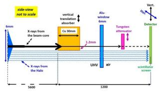
Figure 1: The main components and the paths of the X-rays of both the beam-core and that of the halo population.
