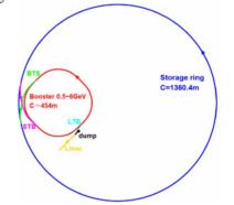
Figure 1: Layout of the HEPS accelerator.
