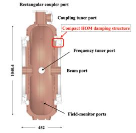
Figure 2: Cross-sectional view of the cavity.
