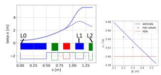
Figure 1: Left:  $\beta_x$  in half UC, regular (line) and for QD=0 (dashed line); magnet color code: MB: blue; RB: purple; QD: red, SF, SD: green. Right:  $\nu_x$ , analytic estimate (blue line), exact phase advance (stars), and option for HOA (red).
