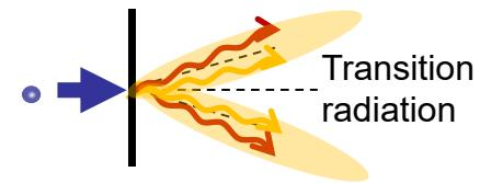
Measure coherent optical transition radiation
