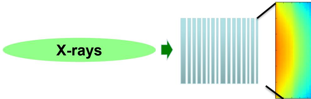
Calorimeter stack layers
