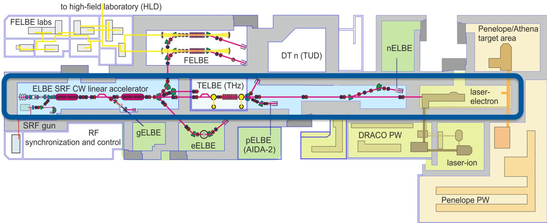
Variable pulse rate (up to 13 MHz) and charge (**up to 0.3 nC**) in 40 MeV ps pulses
