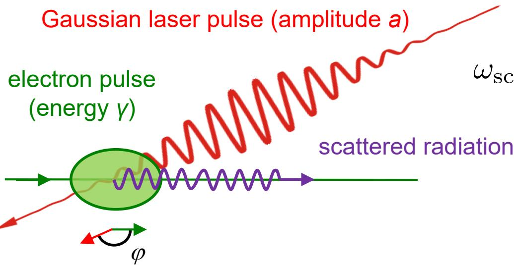
$$\omega_{\text{scatter}} = \frac{2\gamma^2(1 - \cos \varphi)}{1 + \frac{a_0^2}{2} + (\gamma\theta)^2} \omega_{\text{laser}}$$
