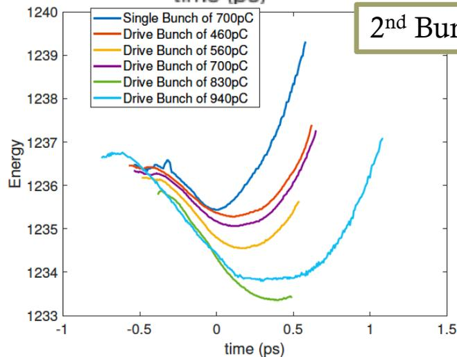
Tuning the **Drive Bunch Charge** allows to manipulate the longitudinal phase space of **Both Bunches**.
