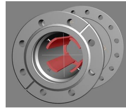
Considering that the signal generated by one bunch takes **1 ns** to reach the short-circuit on a BPM edge and be reflected back, a **2<sup>nd</sup> bunch with  $\Delta T=1\text{ns}$**  perfectly cancels it.
