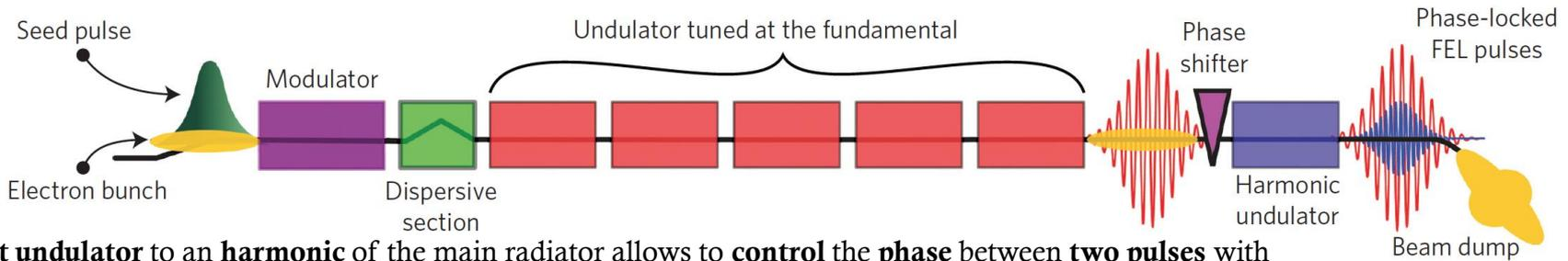
Tuning the **last undulator** to an **harmonic** of the main radiator allows to **control the phase** between **two pulses** with **different wavelength** (with a temporal resolution of **3 attoseconds**).
