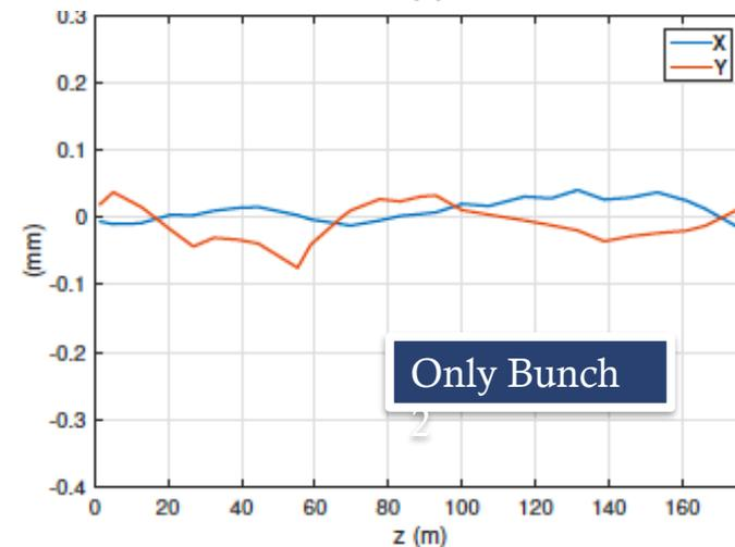
Adjusting the second pulse on the cathode (tens of  $\mu\text{m}$ ) to have no trajectory steering after the gun:
