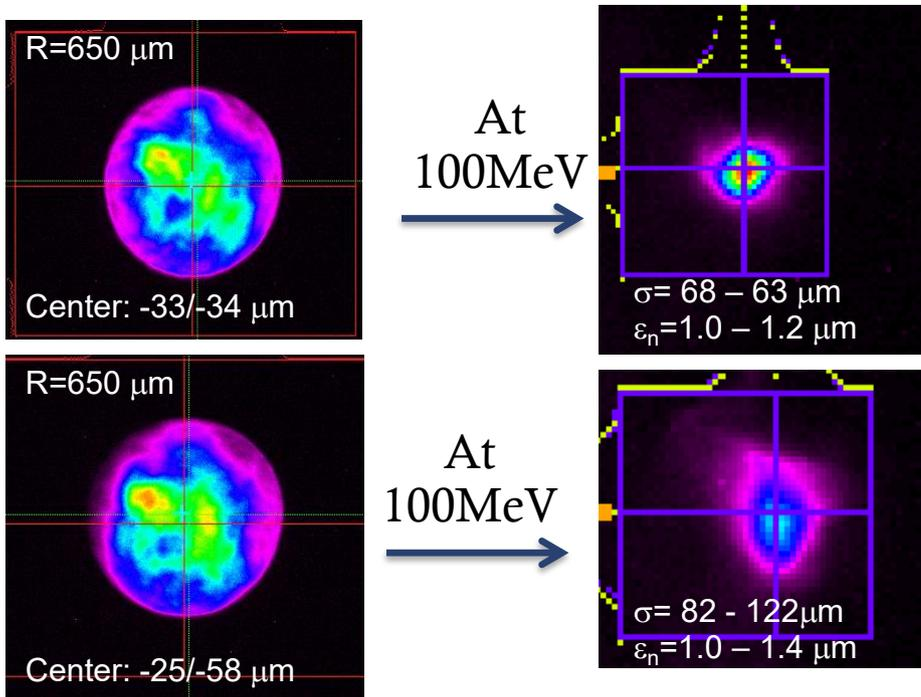
Using the **first bunch trajectory** and **disabling the Feedback**, the second bunch undergoes through a different trajectory already outside the gun
