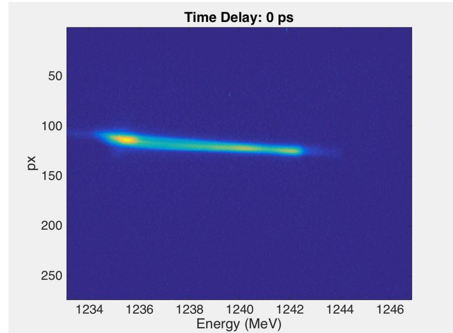
In two-bunch mode also the bunch #1 changes the energy due to the beam loading of the rf linac sections (hard to be compensated in few rf cycles)
