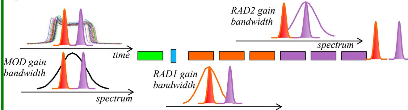
◆ Simultaneous FEL pulses with large ( $>10\%$ )  $\lambda$  separation using single seed with undulators at two harmonics
