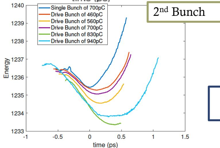
Tuning the **Drive Bunch Charge** allows to manipulate the longitudinal phase space of **Both Bunches**.
