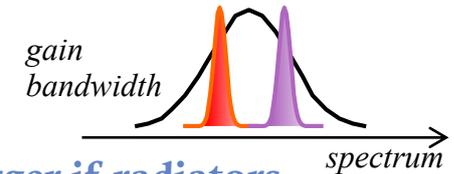
B) FEL Spectral separation 2-3% or larger if radiators are tuned at different harmonics
