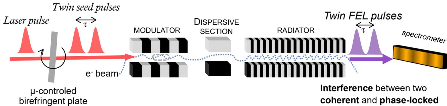
**Two time-delayed seed** pulses are created by transmission of a single laser pulse through a **birefringent plate**. For **coherent pulses**, a fine tuning allows to control the relative phase  $\Delta\phi_{\text{seed}}$
