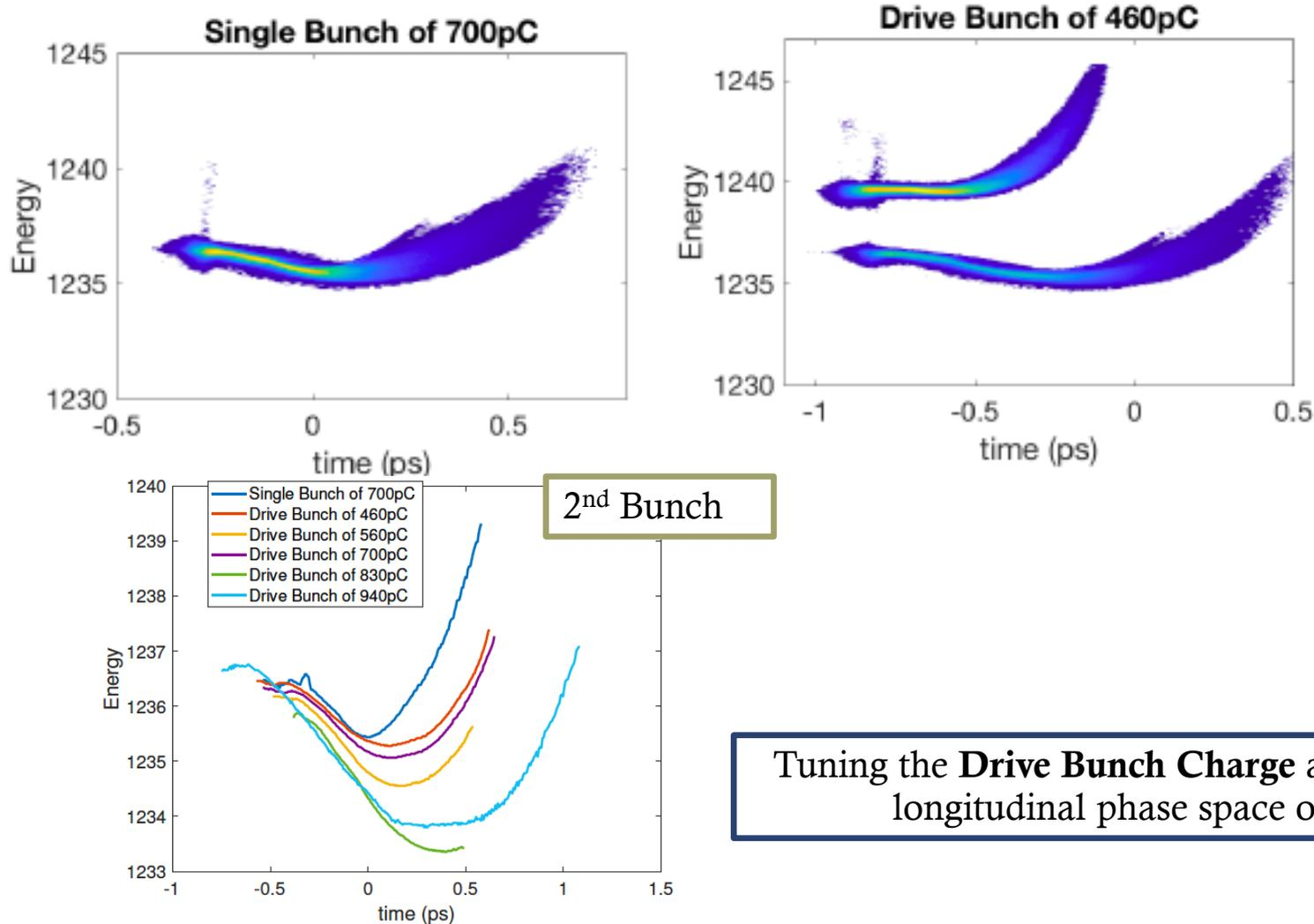
Tuning the **Drive Bunch Charge** allows to manipulate the longitudinal phase space of **Both Bunches**.
