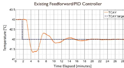
*Note that the oscillations are largely due to the transport delays and water recirculation, rather than PID gains*
