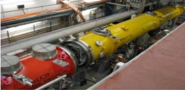
TESLA type superconducting accelerating modules 1.3 GHz
