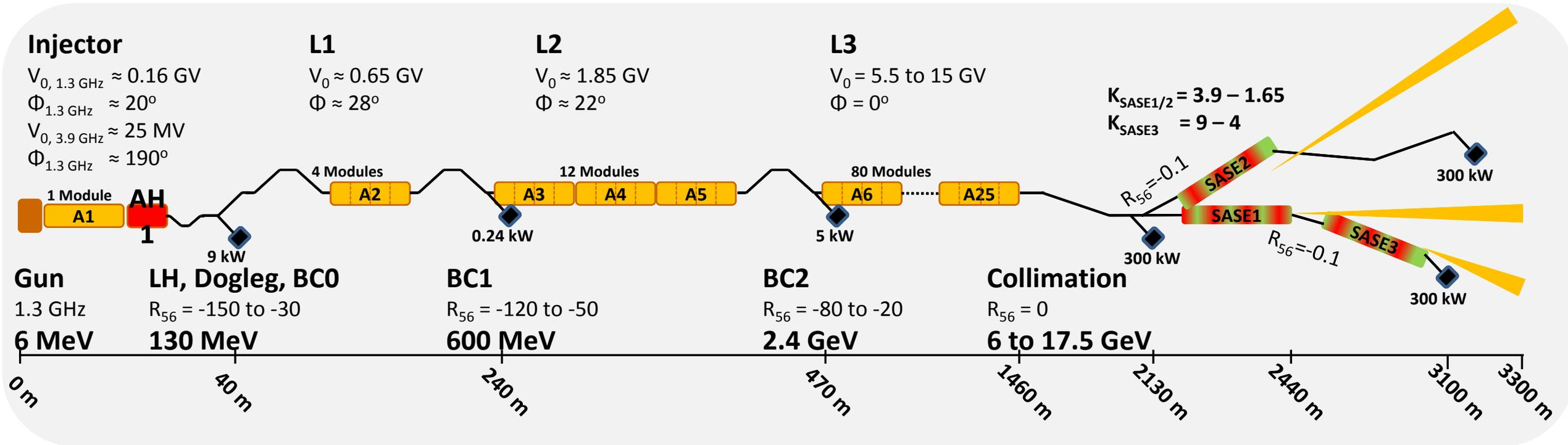
Superconducting linac with 97 1.3 GHz superconducting modules
