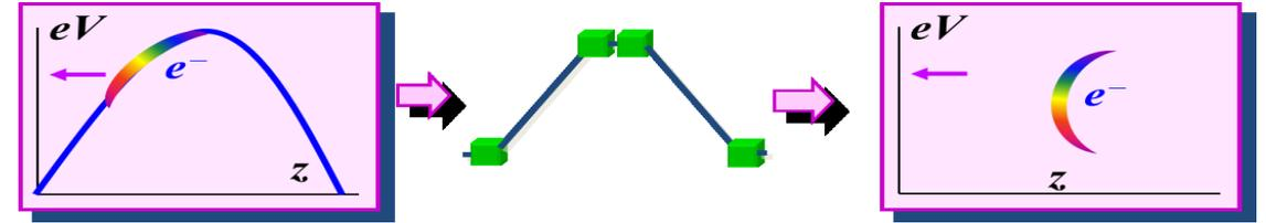
Nonlinear compression produces High density head with low density tail
