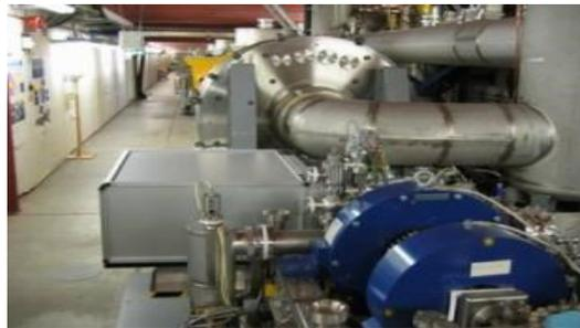
Normal conducting 1.3 GHz RF gun
