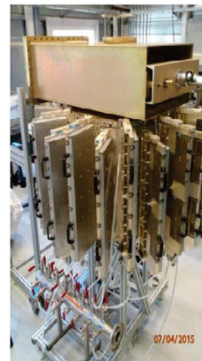
75 kW coaxial power combiner tree
