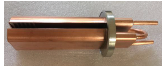
Figure 10: Brazing GlidCop_AL_15 to stainless steel (SST).
