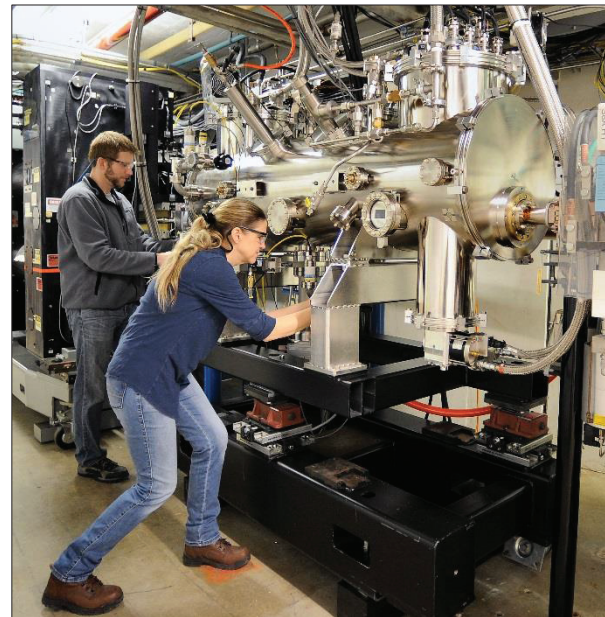
Figure 2: Helical SCU installed in Sector 7.
