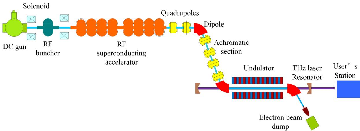
Figure 1: The layout of the CTFEL facility.
