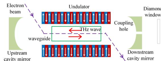
Figure 4: The undulator and the THz optical cavity.
