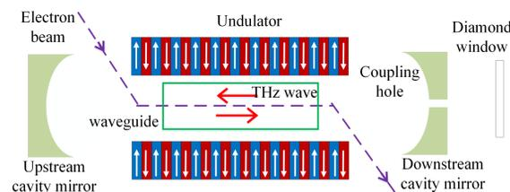
Figure 4: The undulator and the THz optical cavity.
