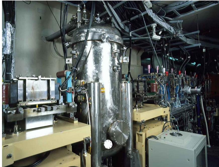
*Superconducting Wavelength Shifter
