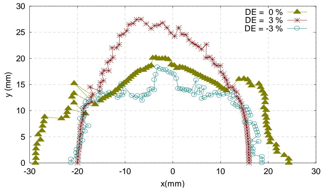
Dynamical aperture for on-energy ad off-energy particles at long straight center
