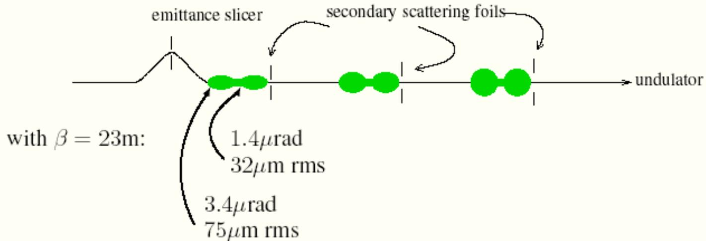
space secondary foils at  $1/2\text{-}\beta$ -function intervals to catch all electrons
