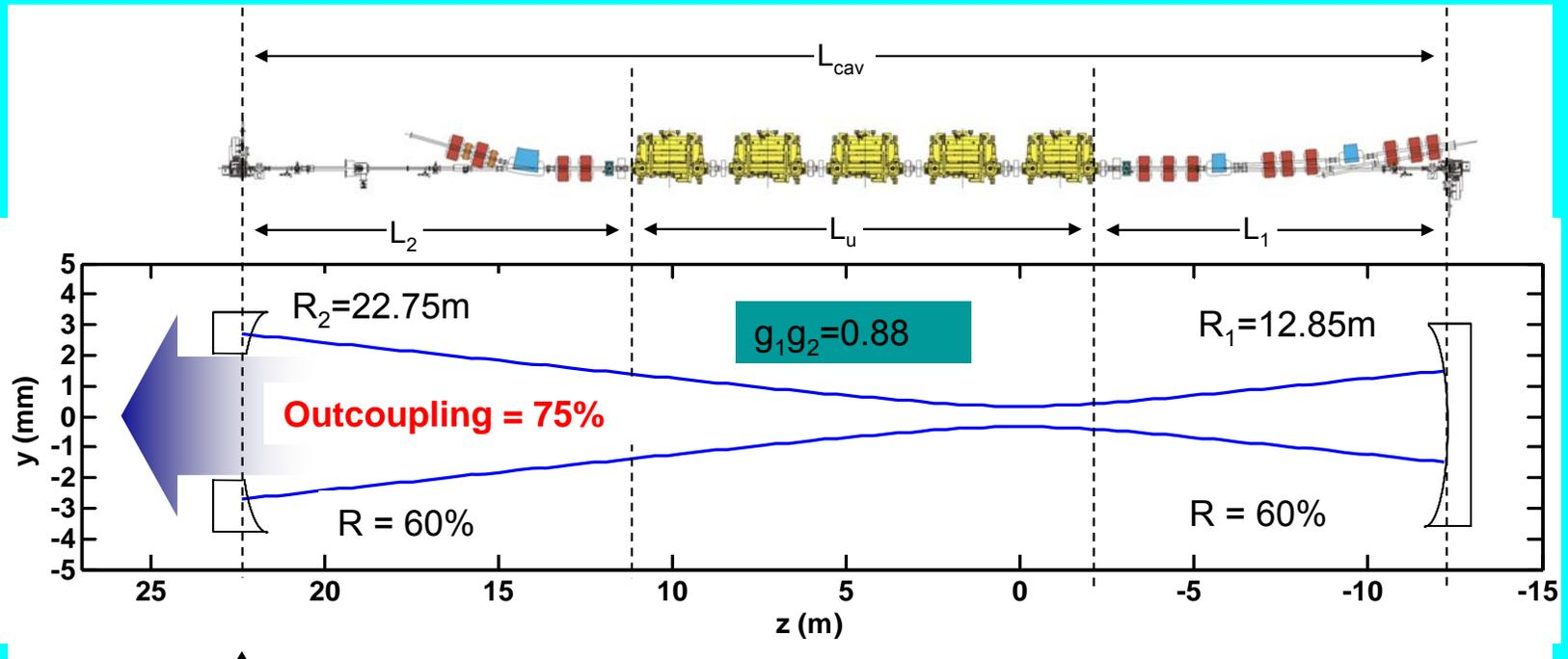
Hole size chosen to be slightly smaller than spontaneous emission spot size on first pass
