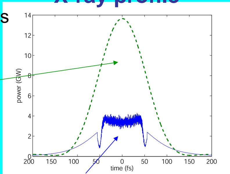
transmitted x-ray (82% transmission for a 100- $\mu$ m diamond)
