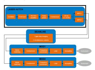
Figure 1: An illustration of the pump-probe laser and its delivery to the experiment.
