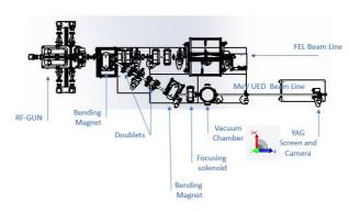
Figure 1: Ariel University's Hybrid Gun. The top beamline is the superradiant THz FEL. The lower beamline is designed for different experiments such as MeV-UED.
