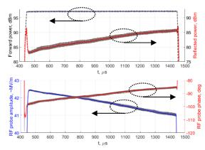
Figure 1: RF signals from 1 ms pulses. Top plot – directional coupler signals. Bottom plot: corresponding RF probe (pickup) signals.
