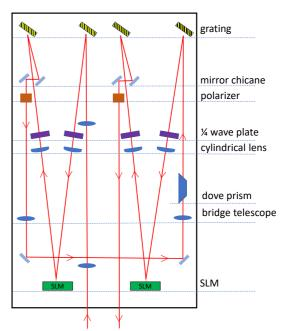
Figure 1: Schematic of a double SLM Shaper.
