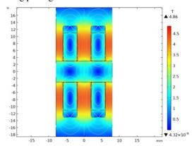
Figure 1: Electromagnetic design of the one period of EuSCU16. A peak field of 4.86 T is reached in the soft iron former at operating current of 500 A. Peak field on axis is 1.5 T.
