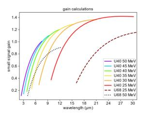
Figure 1: gain calculations for the proposed 40 mm undulator for FEL-2 showing that the  $3-30~\mu m$  region is well covered (solid lines), offer more gain in the  $3-5~\mu m$  region than the 68 mm undulator (dotted line), and maintain good overlap with the highest energy of FEL-1 (dashed line).
