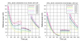
Figure 1: Effect of DFS on reflected power from cavities.
