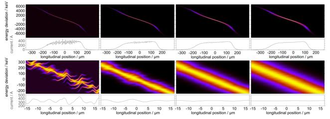
Figure 1: Numerical simulation of the phase space of the full electron beam (top) and the central slice (bottom) together with the current profile at the end of the linac using a recently developed semi-Lagrangian Vlasov simulation code [6]. The images on the left display the situation with the laser heater at zero laser power resulting in an initial sliced energy spread of 3 keV before compression. Towards the right the laser power is increased to reach sliced energy spreads of 5
