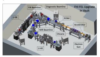
Figure 1: Engineering schematic showing the FHI FEL MIR and FIR electron beamlines in the vault.
