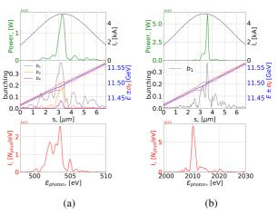
Figure 2: A first part of the FEL is tuned at the fundamental harmonic (a), while a second part lases at the fourth harmonic with respect to the first stage (b). The spikes of the harmonics were effectively filtered when compared to the bunching distribution of the fundamental harmonic. One may observe suppression of low values of bunching, increase in contrast, and reduction of the width of the spike.
