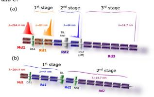
Figure 1: FEL layout (a) FEL-2 in SRC, (b) FEL-2 in HGHG.
