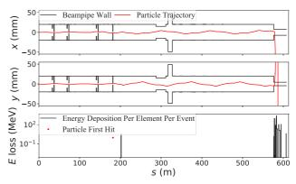
Figure 1: Top and middle plots: trajectory of a particle scattered by a collimator. The particle travels along the following beamline section at large betatron amplitude, before being lost at an aperture reduction near the undulators. Bottom plot: energy deposition by the primary (scattered) particle and by the secondary particles created by the loss of the primary particle.
