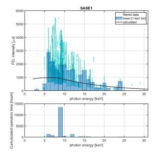
Figure 1: Upper plot: 5-year SASE intensities at SASE1 (cyan dots), and the average value in selected photon ranges (blue bars), compared to calculated intensities for optimized electron energies (black line). Lower plot: Cumulated operation hours within the respective photon energy range.
