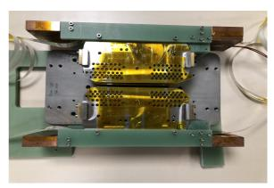
Figure 2: Undulator prototype: structured HTS tape wounded around non-magnetic stainless steel core.
