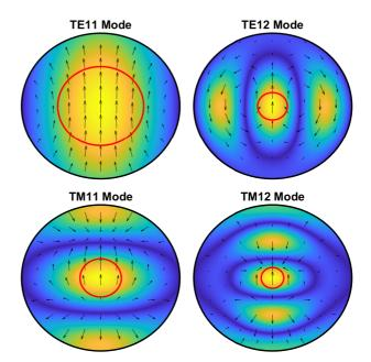
Figure 1: Waveguide Modes. Red circles show electron trajectory and amplitude of  $\vec{v}_z \cdot \vec{E}_{\perp}^{mn}$  is shown by colormap.
