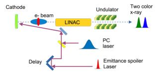
Figure 1: Layout of the two-color FEL scheme based on the laser emittance spoiler.
