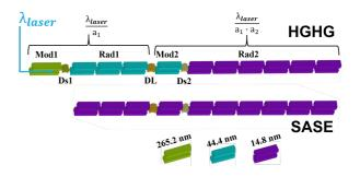
Figure 1: Schematic layout of FERMI FEL-2 operated in cascaded HGHG (top) and SASE (bottom) modes. The undulators are color-coded to the resonant wavelength they were set during the experiment.
