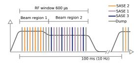
Figure 1: Schematic of the electron bunch distribution to the different SASE beamlines and the dump [1].
