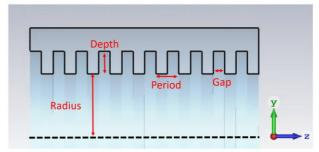
Figure 1: Corrugated beam pipe 2D structure.
