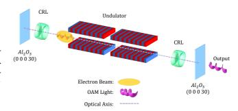
Figure 1: Scheme to generate X-ray OAM beams by using a typical configuration of the XFELO. Compound refractive lenses (CRLs) are used for X-ray focusing.
