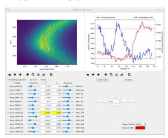
Figure 2: GUI used to monitor the evolution of the spontaneous emission mode while changing the trajectory in the resonant undulator.
