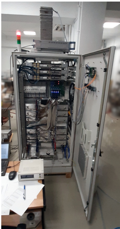
Figure 1: Prototype of the solid state amplifier for PolFEL under development.
