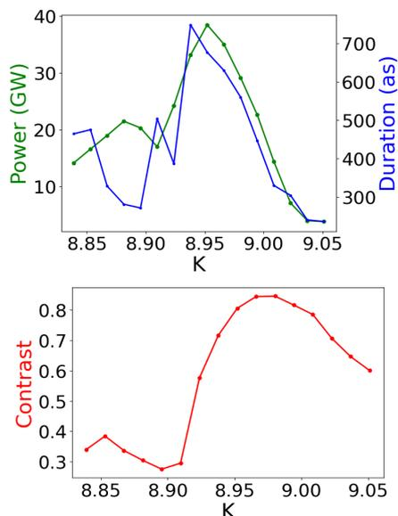
Figure 8: Scanning of the undulator strength of the second stage.
