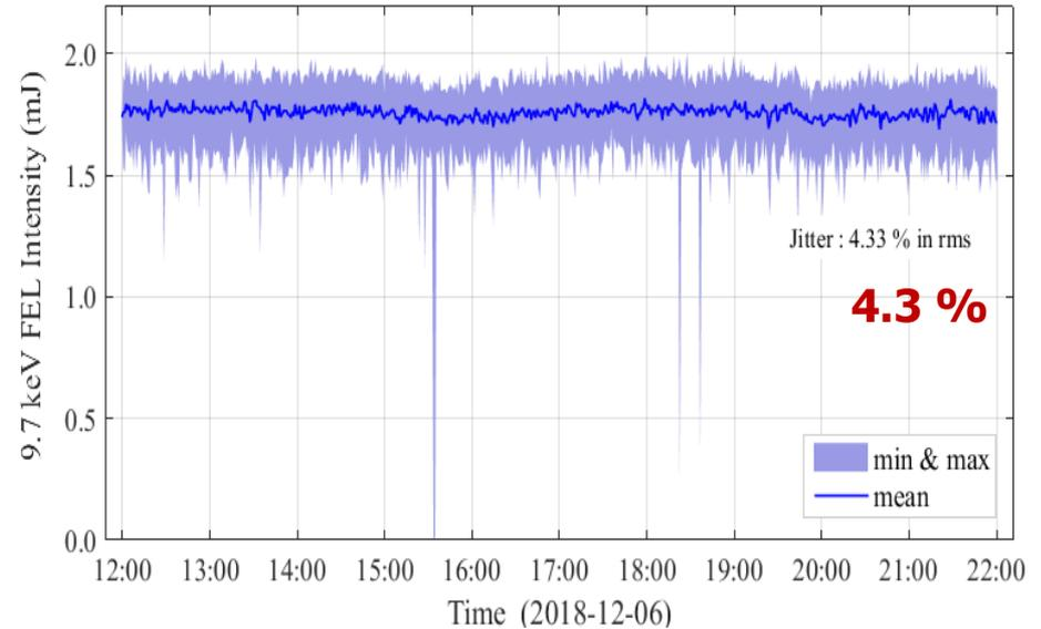
Fluctuations of the radiation pulse energy at the end of the exponential gain regime
